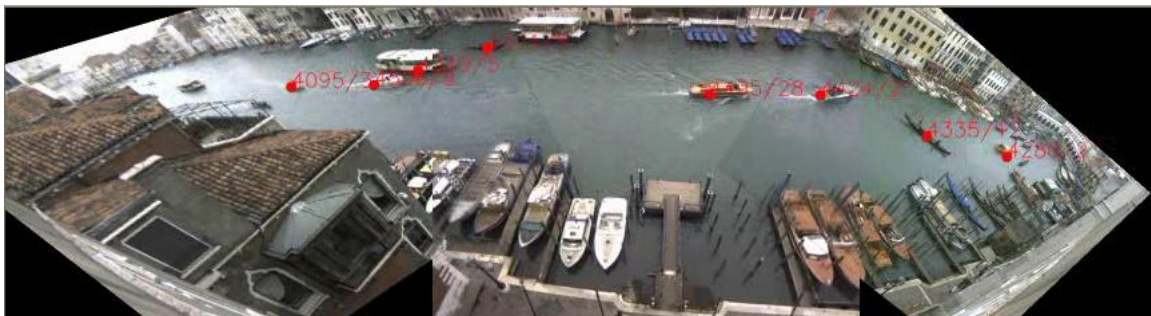
Figure 9: With the ARGOS system, live images are stitched together to generate a view of the Grand Canal. Observations are used from a multi-step Kalman filter to track targets over time 3
