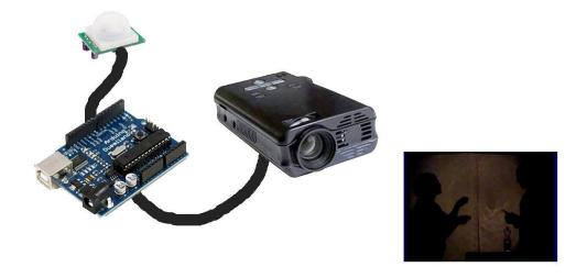
Figure 61 - Pico Projector activated by PIR motion sensor
