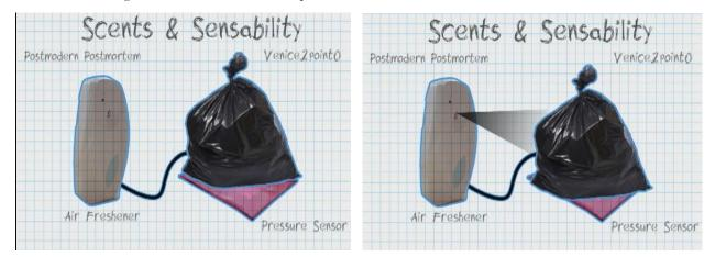
Figure 1 - Trash Bag is Place on the Sensor, Air Freshener Sprays a Few Seconds Later
