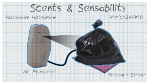
Figure 59 - Air freshener sprays when the trash is detected
