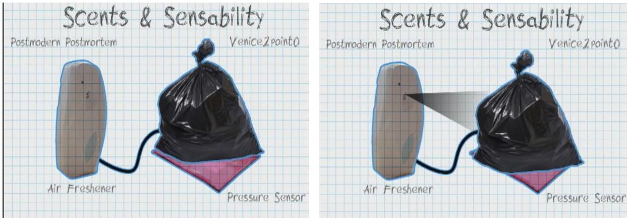
Figure 1 - Trash Bag is Place on the Sensor, Air Freshener Sprays a Few Seconds Later
