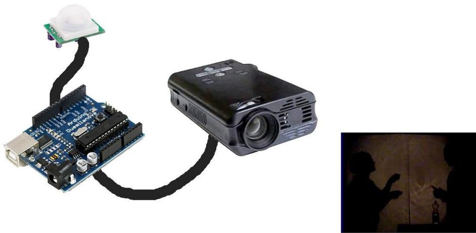
Figure 61 - Pico Projector activated by PIR motion sensor
