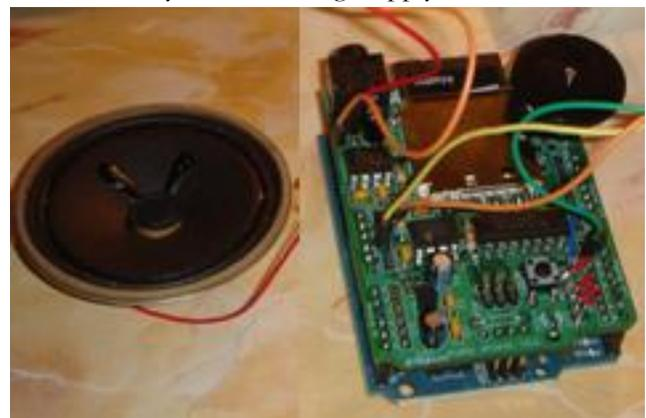
Figure 18 - Arduino with Wave Shield and Speaker
