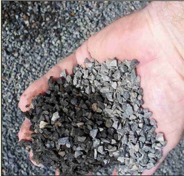
Figure 132: Close—Up of Crushed Gravel 59
