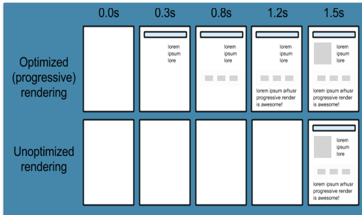
Figure 2: Critical Rendering Path - Optimized rendering vs Unoptimized rendering
