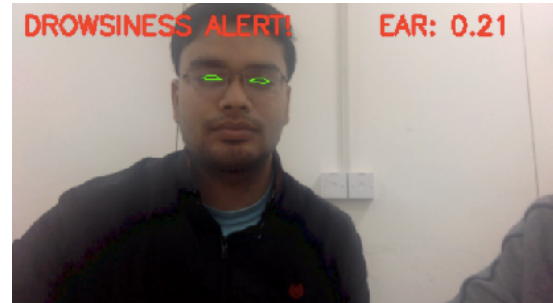
Figure 19: A team member being warned of drowsiness using our eye detection system on April 3, 2018
