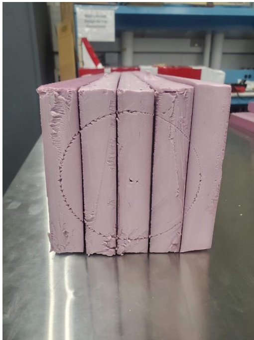
Figure 38: Face of the cut foam board, scored to see necessary shape and dimensions of the resulting cylinder
