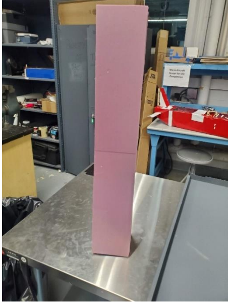
Figure 36: Foam board cut to the width needed for the fuselage
