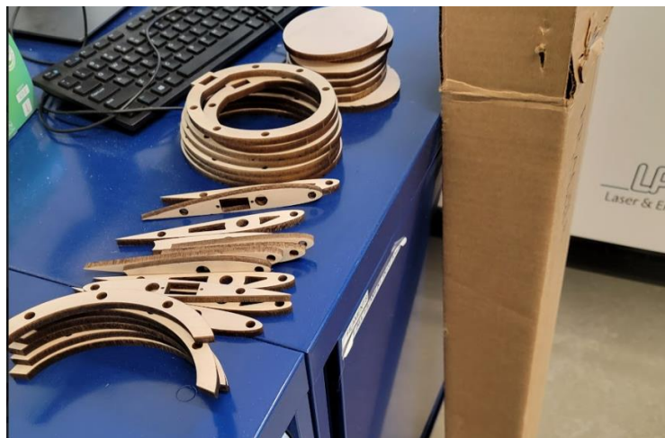
Figure 42: Laser Cut Fuselage and Wing ribs
