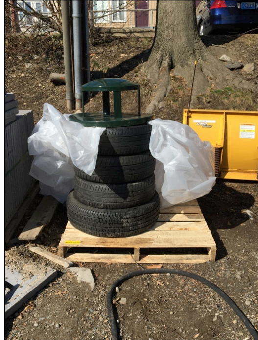
Figure 34: Tire tank with metal garbage can cover at the end of the 3 week trial period
