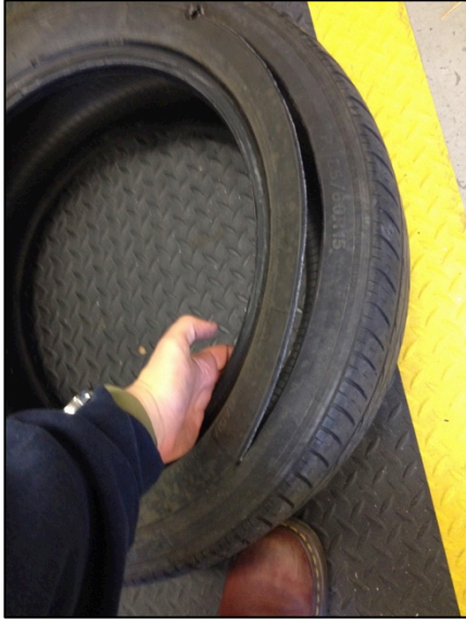
Figure 28: Tire cut with jig saw
