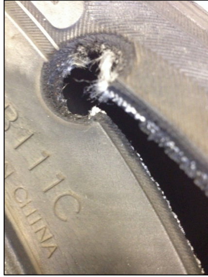
Figure 29: Tires have steel mesh under layers of rubber
