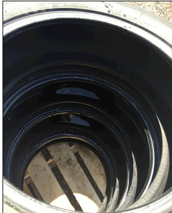
Figure 36: Water condensed on the outside of the plastic and pooled in the tire rims
