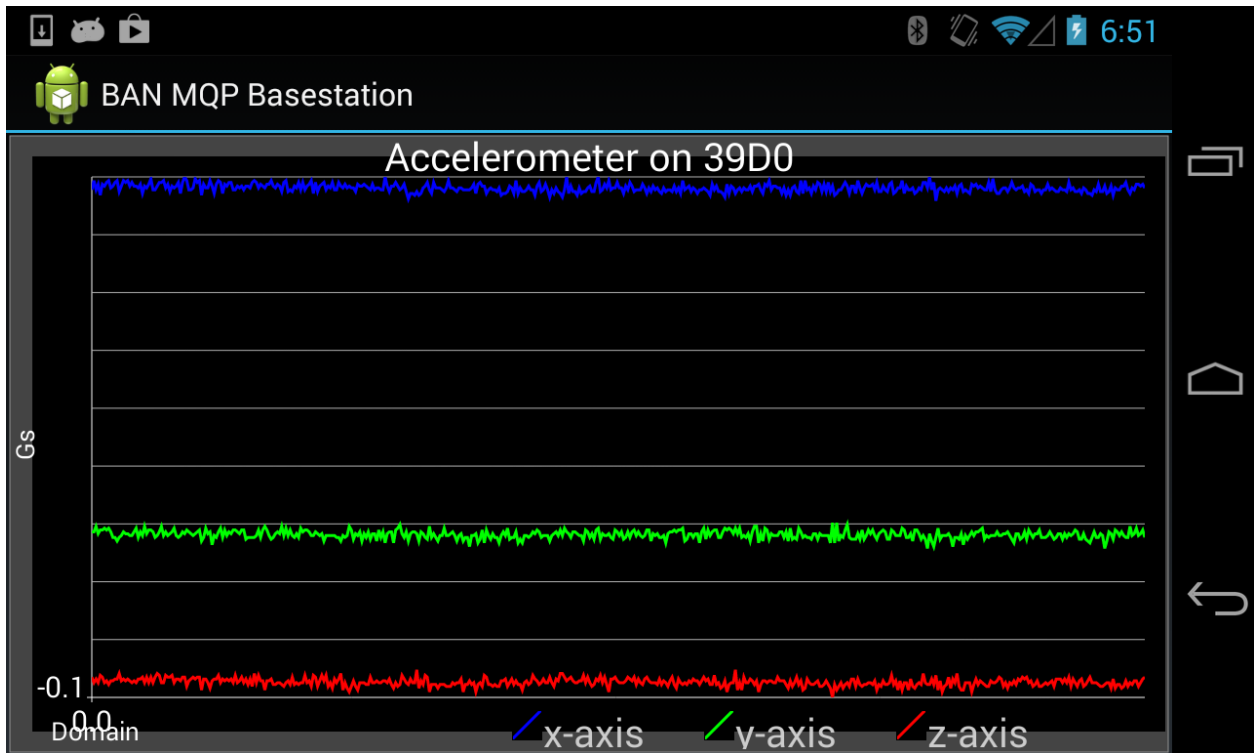
Figure 36: Base Station Application Graphing Resting 3-Axis Accelerometer
