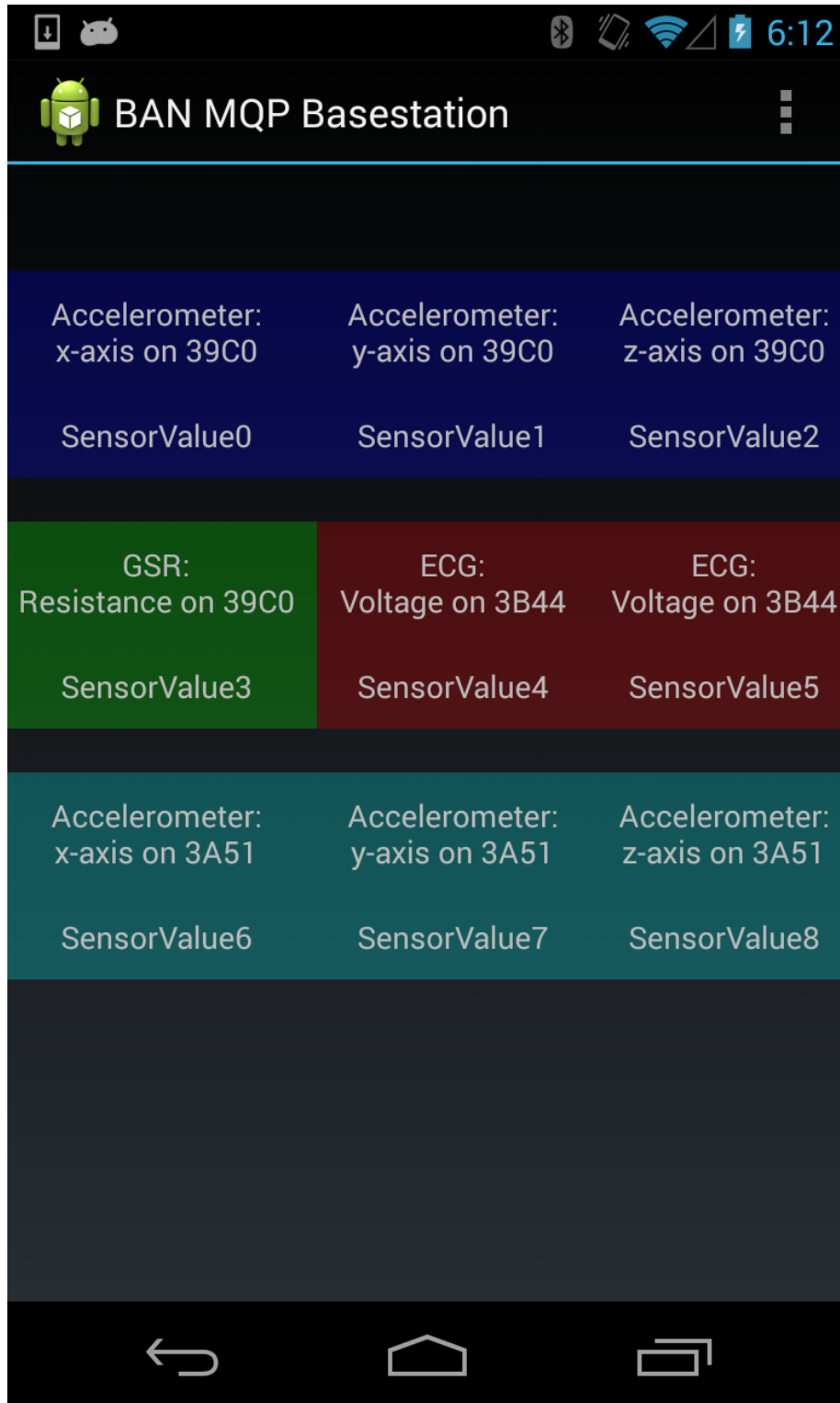
Figure 34: Base Station Application With Three Motes Added
