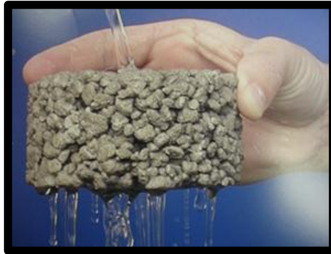
Figure 14: Porous Concrete Demonstration
