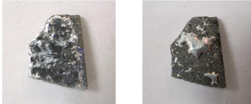
Figure 9.3 SiC-Ga-1wt%Mg wettability coupon tests before (left) and after heating (right).
