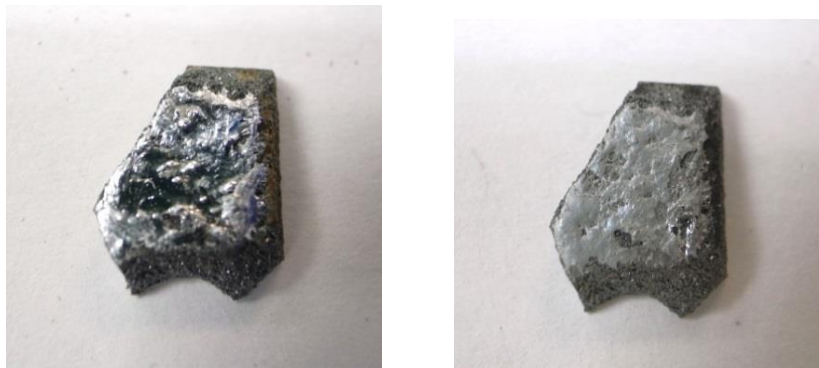
Figure 9.4 SiC-Ga-2wt%Mg wettability coupon tests before (left) and after heating (right).
