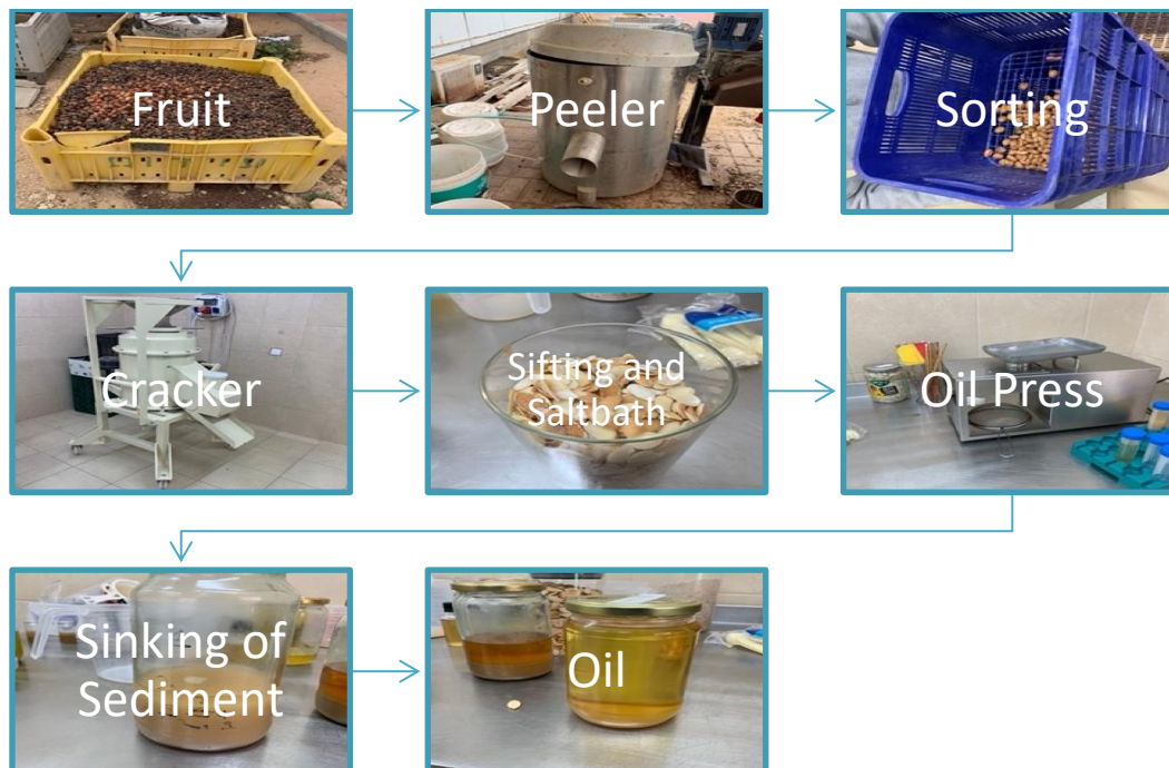
Figure 1.1: Kibbutz Ketura's Argan Oil Process
