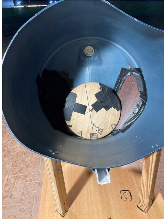
Figure 3.6: Image of the Rotating Plate in the Feeder System
