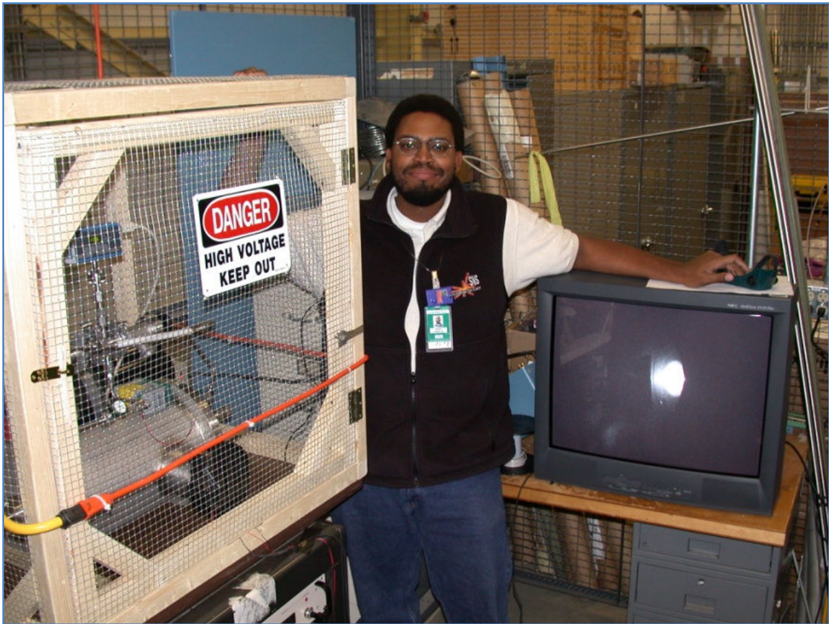
Figure 5.3 - Plasma source test stand and graduate student Jerry Carr Jr. The vacuum chamber which tests the plasma gun can be seen inside the faraday cage. The ion gauge and camera can also be seen, along with the video seen on the television of the operational plasma gun.
