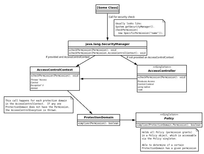
Figure 1.1: Control flow of a typical security check
