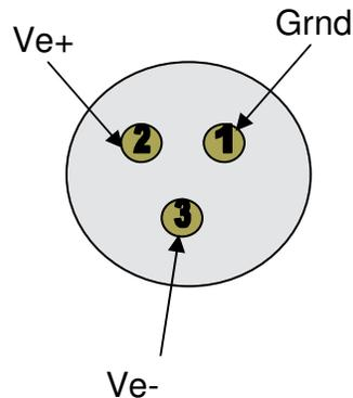
**Figure 2.1: XLR connector numbering.**
