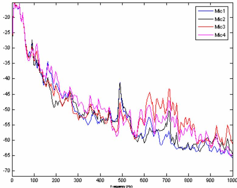
**Figure 4.23: Driving 30 MPH normalized 0-1 kHz PSD.**
