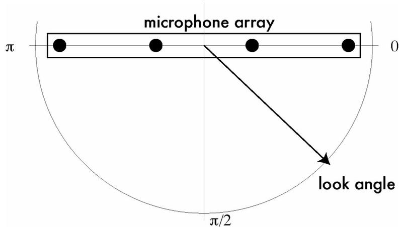
**Figure 2.4: Microphone array.**
