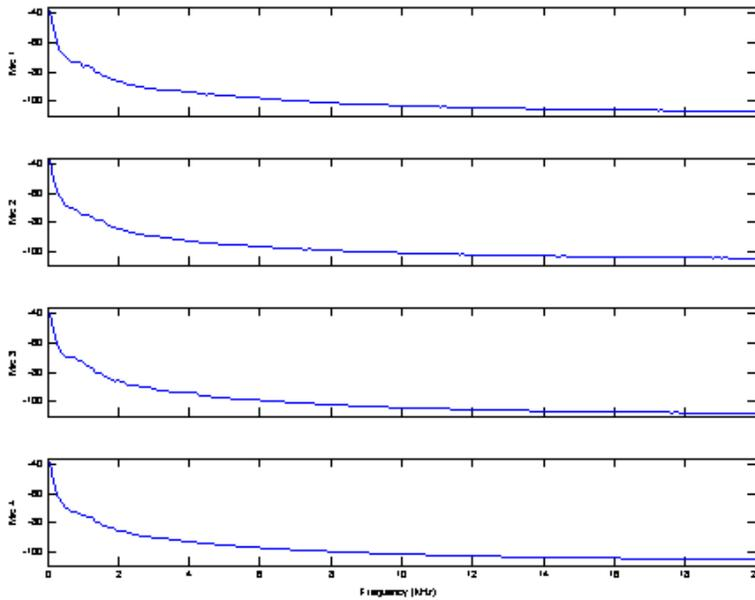
Figure 6.2. Normalized PSD 0-20kHz, Amplitude in dB
