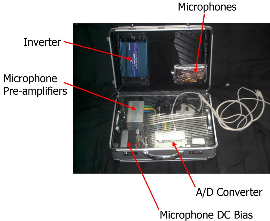
**Figure 3.3: Mechanical layout of the suitcase.**
