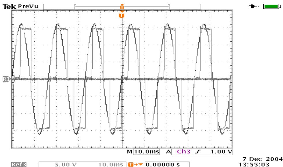
Figure 2.3: Modified sine wave vs. pure sine wave.
