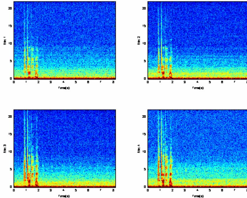
**Figure 4.15: Car idle 0-20 kHz spectrogram.**
