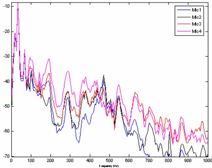
**Figure 4.14: Car idle normalized 0-1 kHz PSD.**
