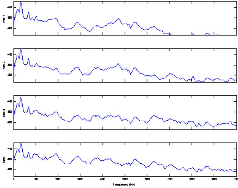
Figure 3.4. Normalized PSD 0-1kHz, Amplitude in dB
