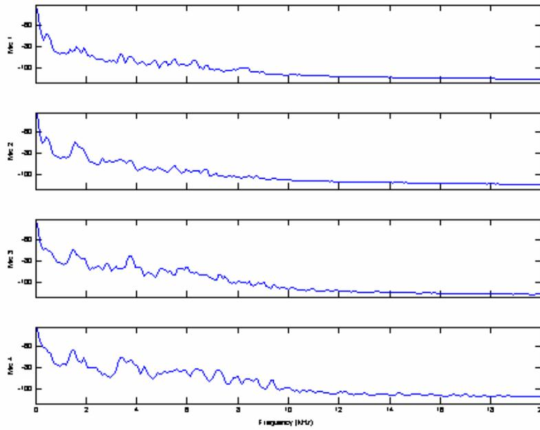
**Figure 4.11: Jeep car idle non-normalized 0-20 kHz PSD.**
