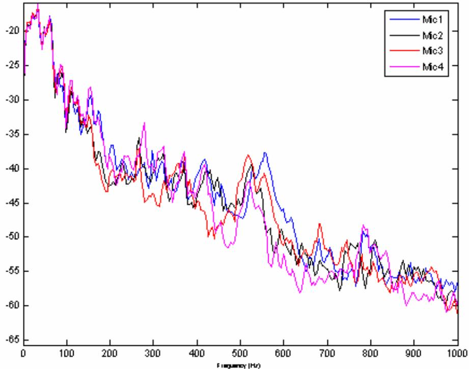
**Figure 4.25: Accelerating 30-50 MPH normalized 0-1 kHz PSD.**
