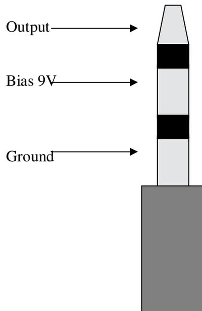
**Figure 2.2: Breakdown of a TRS plug.**
