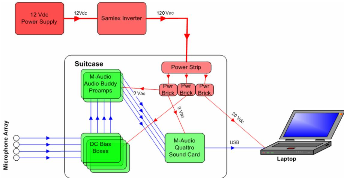
**Figure 3.2: Signal and power flow diagram.**
