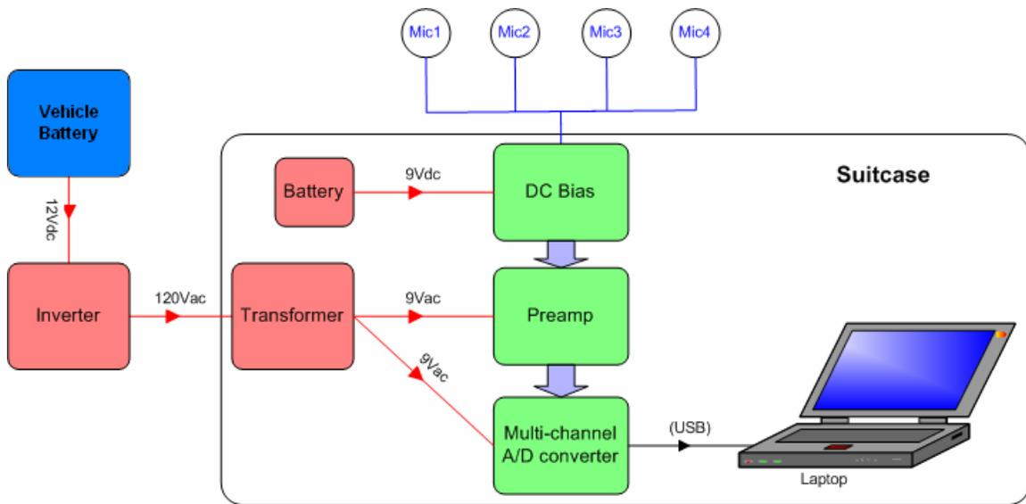
Figure 3.1: Hardware block diagram.
