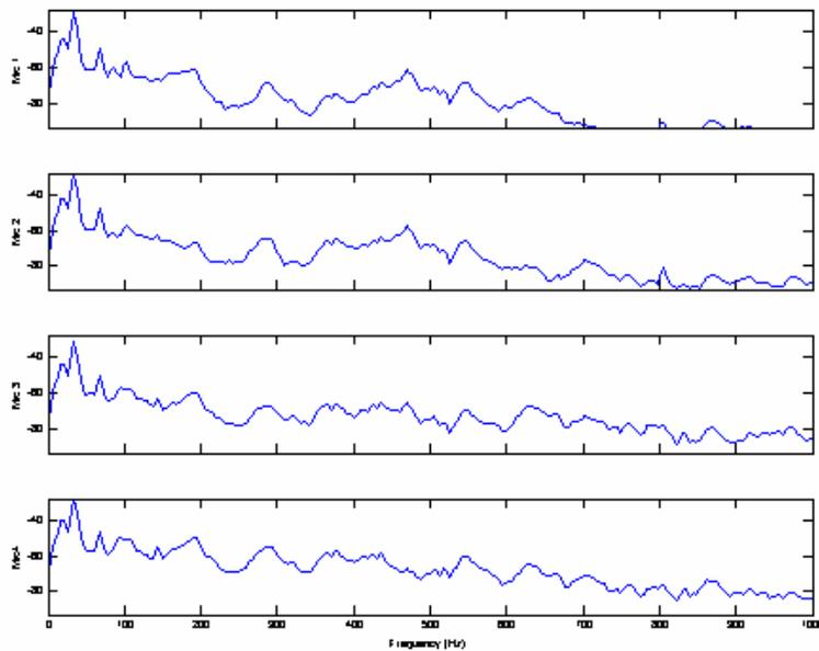
**Figure 4.12: Car idle normalized 0-1 kHz PSD.**
