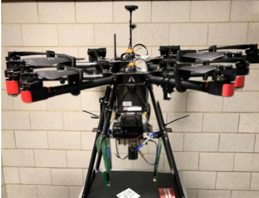
*Figure 3.4.1 Aurelia X6 Max Drone with Radar mounted*
