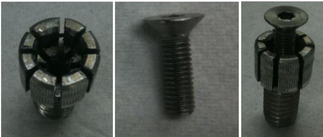
**Figure 26: Manufactured outer screw, inner screw, and assembly prototypes.**
