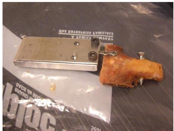
**Step 4:** The custom grip is attached to the upper Instron grip and an endcap with epoxy is filled and attached to the lower Instron grip. The Instron grip is then lowered into the epoxy to make sure the sample is aligned.
