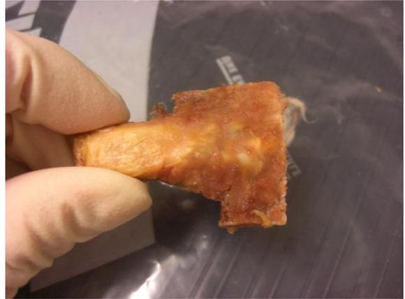
**Step 2:** Two holes are drilled into the sternum segments as shown. The sternum is kept in the ziplock bag to contain any biohazardous material. Another hole is drilled into the side of the rib segment for the anchoring screw.
