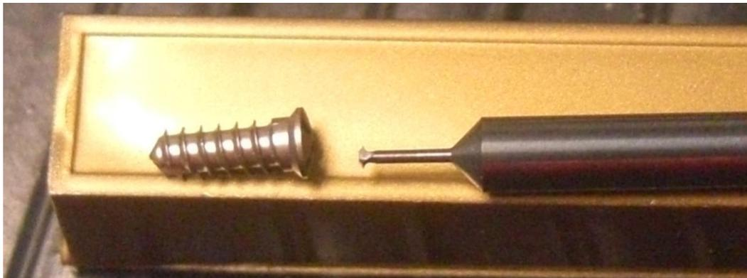
Figure 34: Screw and Thread mill close-up.
