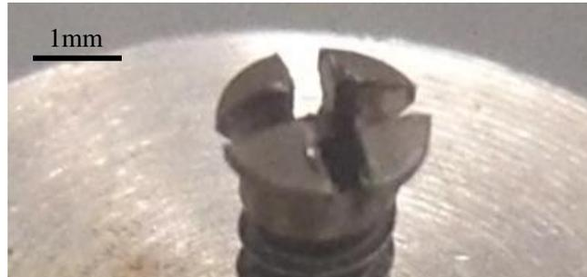
Figure 36: Close-up view of expansion slits that were cut using wire EDM.
