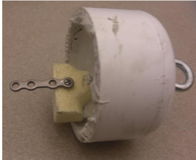
**Figure 22: Setup of sample fixed in PVC endcap with eyehook.**
