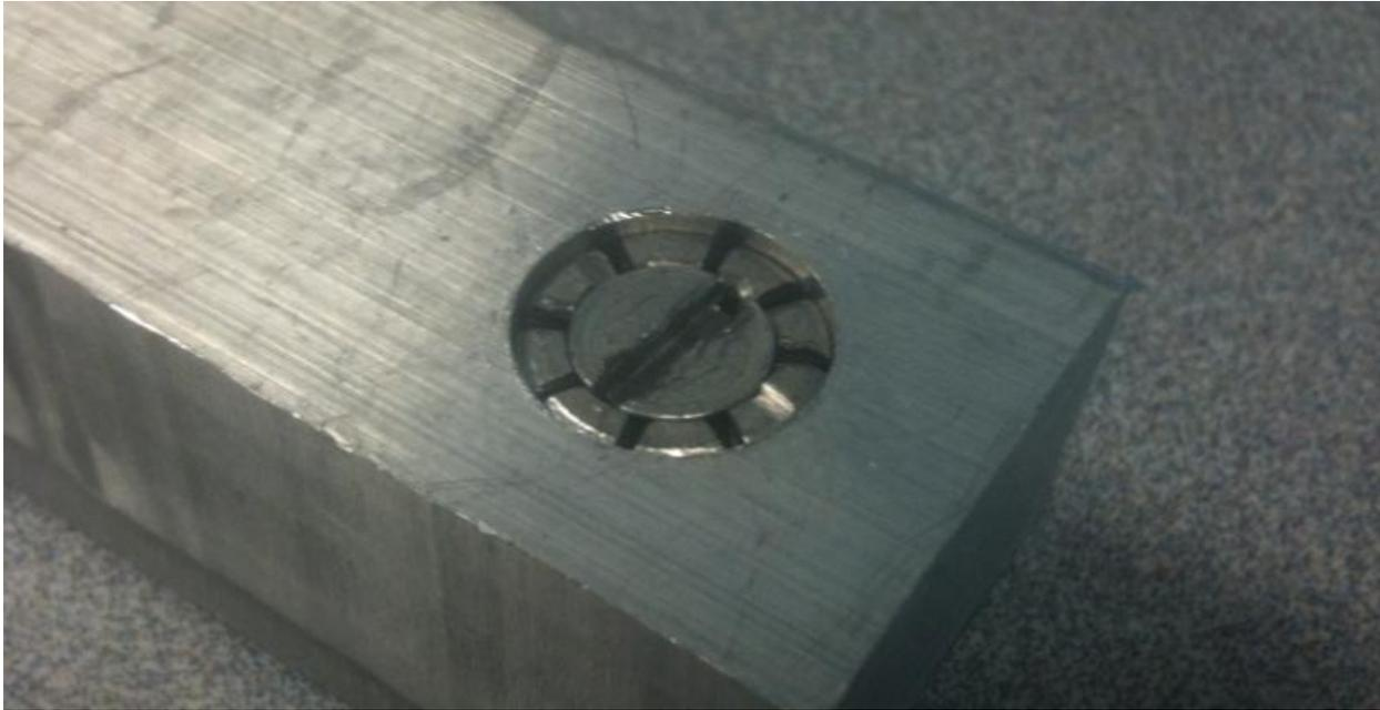
**Figure 28: Validation of the locking mechanism. Inner screw has been tightened and the head of the outer screw has engaged the plate. After removal of the bone plate from below, blunt forces to the screw thread post did not dislodge the part.**
