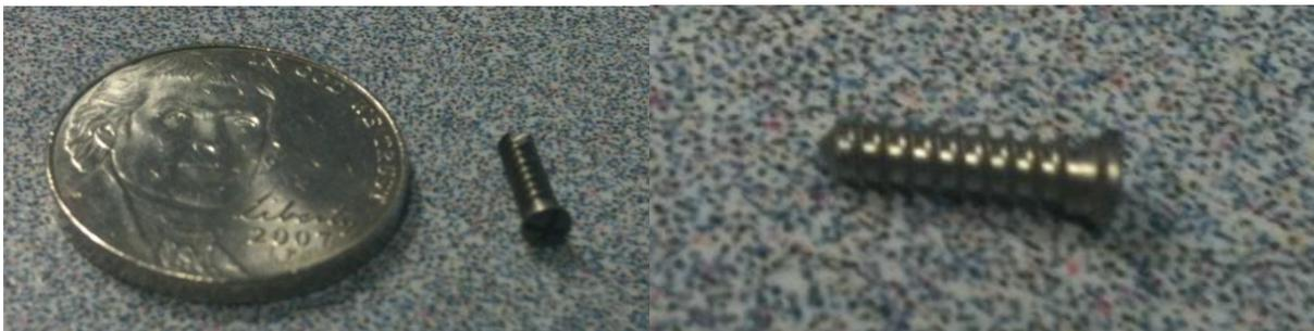
**Figure 29: KLS Martin screw adjacent to a nickel (left) and a close-up of the thread pattern and head profile (right).**
