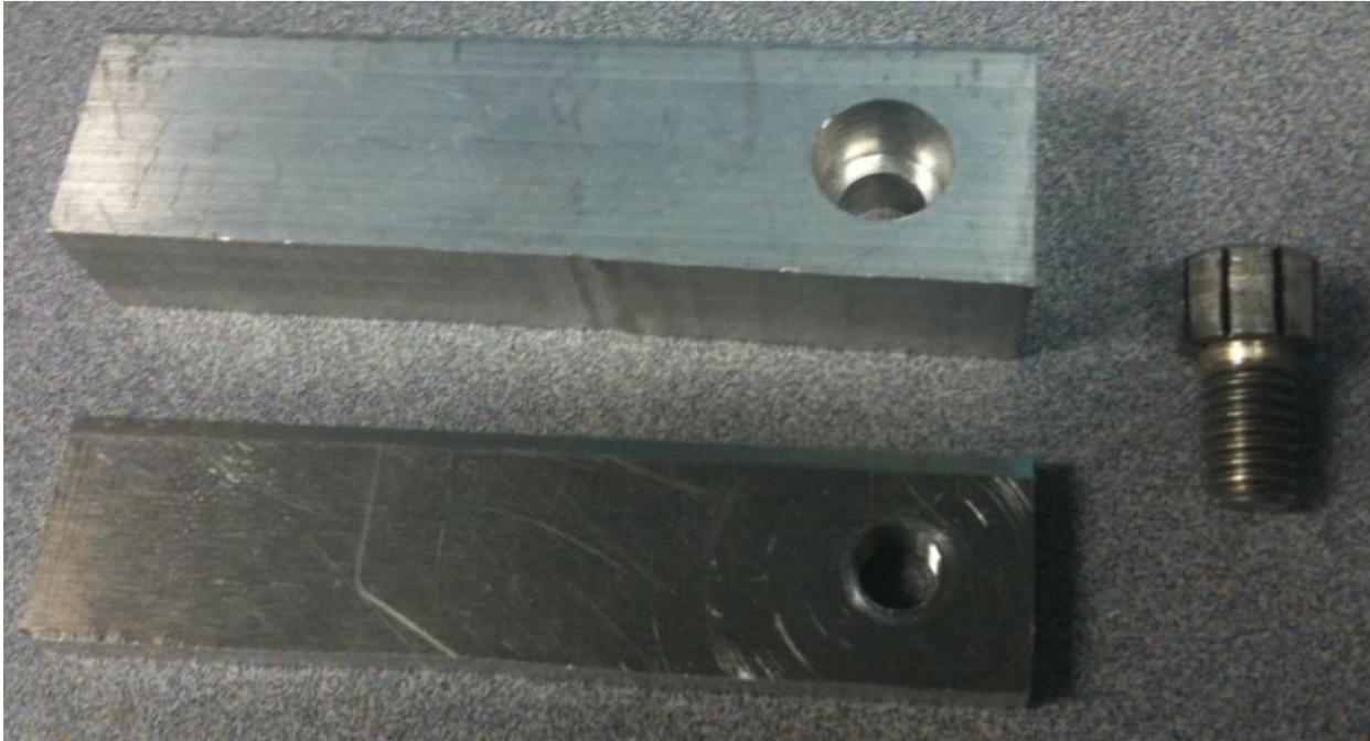
**Figure 27: Milled plate (top), threaded bone plate (bottom), screw assembly (right).**
