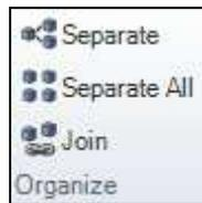
Figure 49: SpaceClaim Tools for Joining and Separating Two Shells. Original Drawing in SpaceClaim
