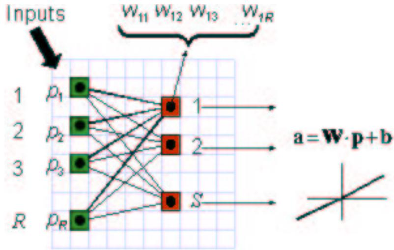
Figure 4.13: The ADALINE neural network.  $p$  refers to the matrix of input vectors.  $R$  refers to the number of inputs to the input layer.  $W$  is the weight matrix.  $b$  represents the bias vector.  $S$  is the number of neurons in the output layer. The plot in the lower right corner of the figure illustrates the linear training function. In the small graph to the right, the x-axis represents the input,  $p$  and the y-axis represents the output,  $a$ .
