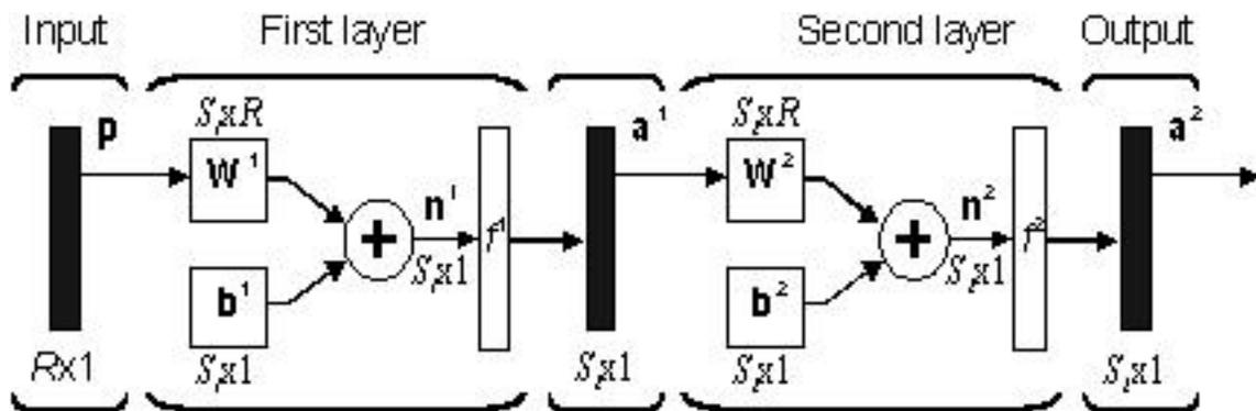
Figure 4.14: The backpropagation neural network.  $R$  refers to the number of inputs to the input layer.  $S$  refers to the number of neurons in the output layer.  $P$  is the matrix of input vectors ( $R \times$  the number of training pairs).  $W$  is the weight matrix and  $b$  refers to the bias vector.  $n$  is the matrix of values output from the first layer of neurons.  $f$  refers to the transfer function.  $a$  indicates the matrix of output vectors.
