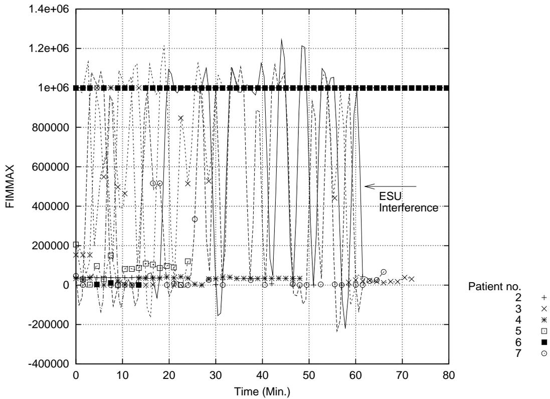
Figure 8.5: *FIMMAX* (frequency of minimum reactance) data contaminated with ESU interference. This figure presents the data from patients two through seven. Note the spikes caused by ESU contamination.
