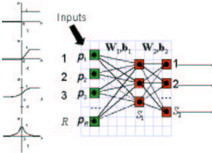
Figure 4.15: The backpropagation neural network and transfer functions. The row of plots on the left hand side of the diagram illustrate the possible transfer functions that can be used with a backpropagation neural network. For these plots, the x-axis refers to the input,  $p$ , and the y-axis represents the output,  $a$ . Refer to Figure 4.13 for the definition of variables seen in the figure.
