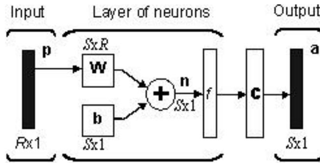
Figure 4.12: The Hebbian neural network.  $R$  refers to the number of inputs to the input layer.  $S$  refers to the number of neurons in the output layer.  $P$  is the matrix of input vectors ( $R \times$  the number of training pairs).  $W$  is the weight matrix and  $b$  refers to the bias vector.  $n$  is the matrix of values output from the first layer of neurons.  $f$  refers to the transfer function.  $c$  represents the competitive layer.  $a$  indicates the matrix of output vectors.
