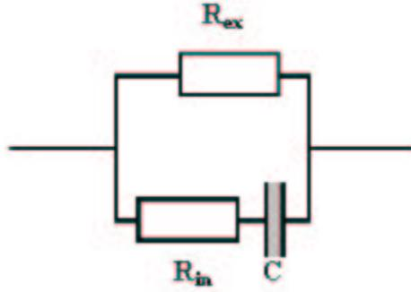
Figure 4.1: Electrical model of biological tissue where  $R_{ex}$  represents the resistance of the extracellular space,  $R_{in}$  represents the resistance of the intracellular space and  $C$  represents the membrane pseudo-capacitance.
