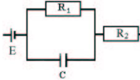
Figure 4.6: The electrical model of the electrode-electrolyte interface.  $E$  represents the half-cell potential. The  $R_1$  and  $C$  parallel combination represent the electrode-electrolyte interface and  $R_2$  represents the electrolyte resistance.
