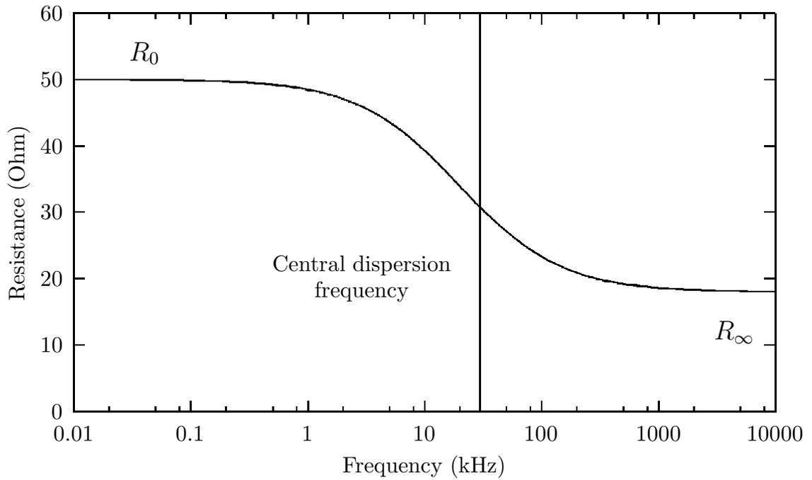
Figure 4.3: A typical plot of tissue resistance  $Re\{Z\}$  against frequency using the electrical model illustrated in Figure 4.1.  $R_0$  refers to the resistance measured at 0 frequency.  $R_\infty$  refers to the resistance at very high frequencies. The central dispersion frequency is illustrated. Please note that this is for the  $\beta$  dispersion region.
