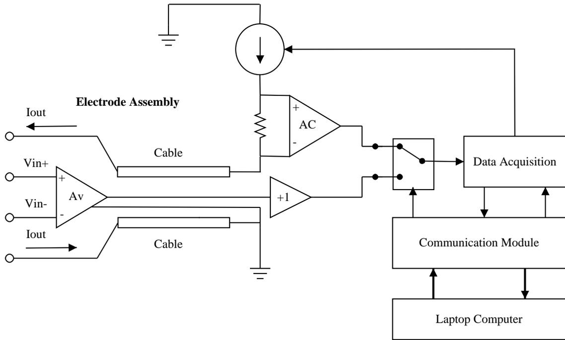
Figure 4.10: Detailed diagram of the electrode assembly and its connection to the impedance spectrometer (IS) [5].  $I_{out}$  refers to the current output from the instrument and injected into the tissue.  $V_{in}$  refers to the voltage recorded from the tissue. The electrode assembly further consists of an instrumentation amplifier and a cable with a driven shield.
