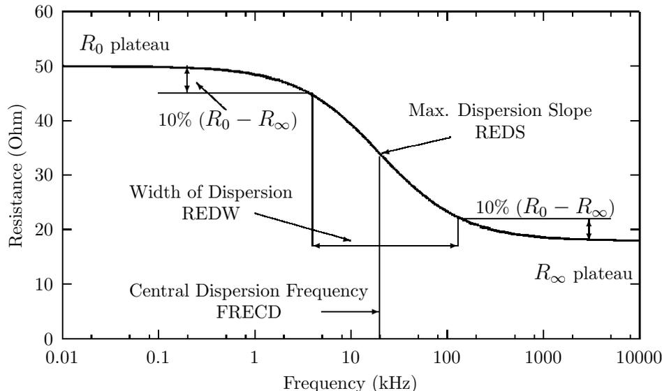
Figure 9.3: The resistance curve parameters. The parameters illustrated are:  $R_0$ ,  $R_\infty$ , REDS, REDW, and FRECD.
