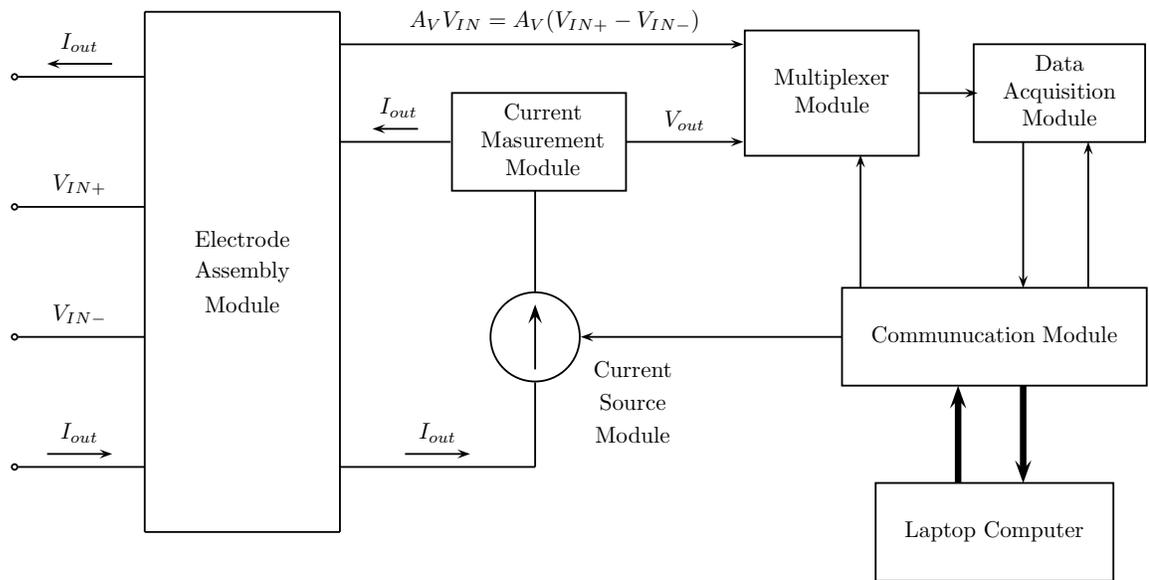
Figure 4.9: A block diagram of the impedance spectrometer [5].  $I_{out}$  refers to the current output from the instrument and injected into the tissue.  $V_{IN}$  refers to the voltage recorded from the tissue. The unit physically consists of three parts. The electrode assembly (electrodes and cable configuration), the impedance spectrometer (current measurement, multiplexor, current source, data acquisition, and communication modules) and the laptop that controls the impedance spectrometer.
