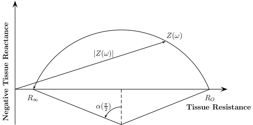
Figure 4.2: A typical Nyquist plot with the negative tissue reactance  $-Im\{Z\}$  plotted against the tissue resistance  $Re\{Z\}$ .  $R_0$  refers to the resistance measured at 0 frequency.  $R_\infty$  refers to the resistance at very high frequencies.  $Z(\omega)$  refers to the impedance as a function of frequency and  $|Z(\omega)|$  refers to the magnitude of the impedance.  $\alpha(\pi/2)$  is related to the depression of the center of the locus.
