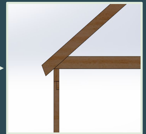
Modified Truss Overhand to Provide Robust Fixturing
