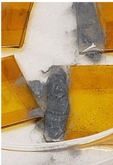
Figure 17: Reaction of Zinc Powder and HCl Solution on the Glass Cell
