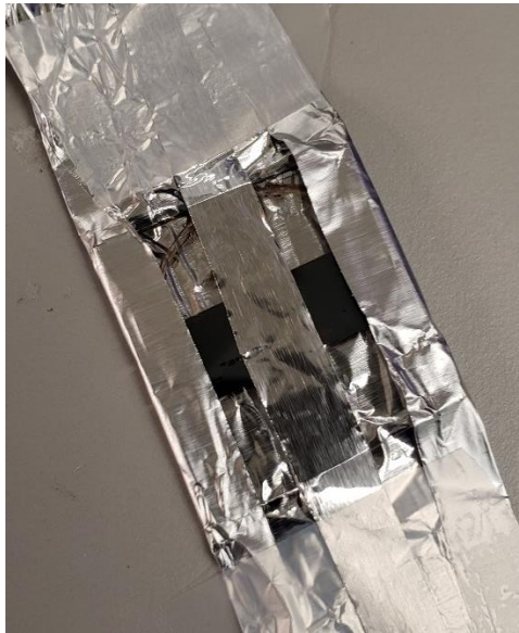
Figure 21: Cell Prepared for Gold Deposition
