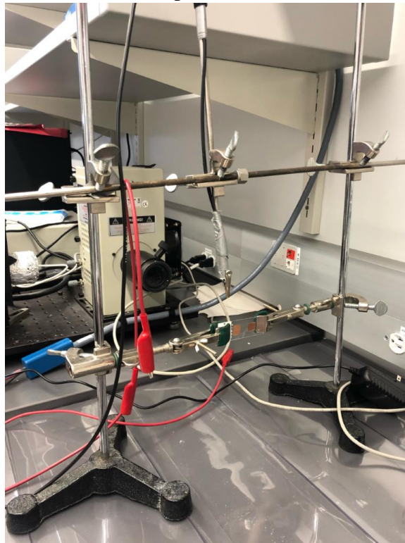
Figure 23: The JV Curve Testing Apparatus
