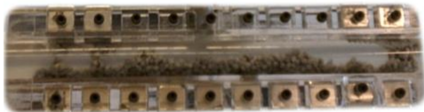
Figure 26: Beads held in place by magnetic field
