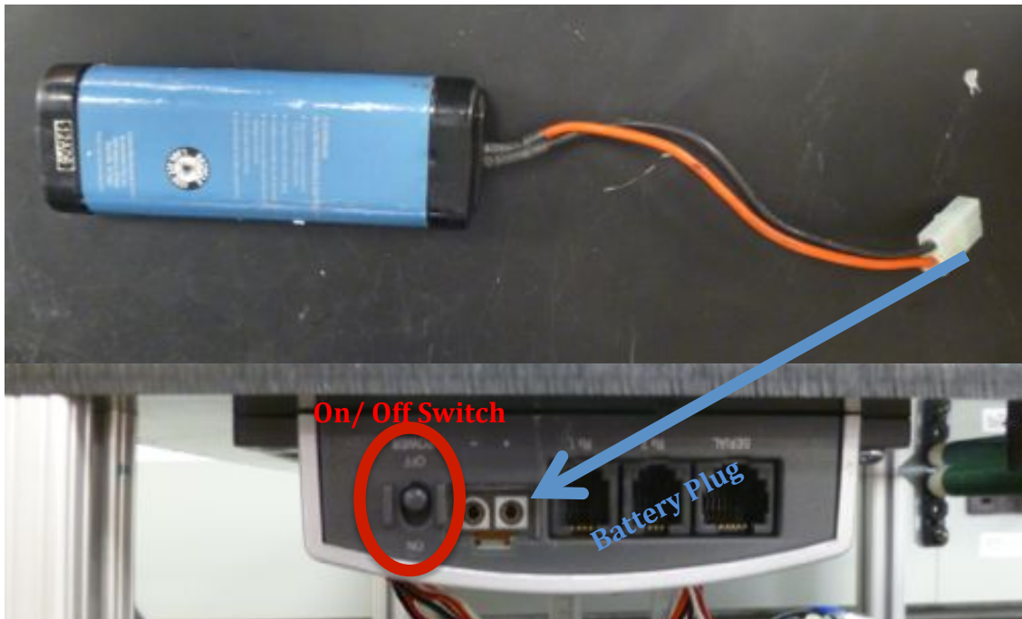
Figure 79: Battery Insertion - above is the battery and where to plug it into the microcontroller, as well as the on switch
