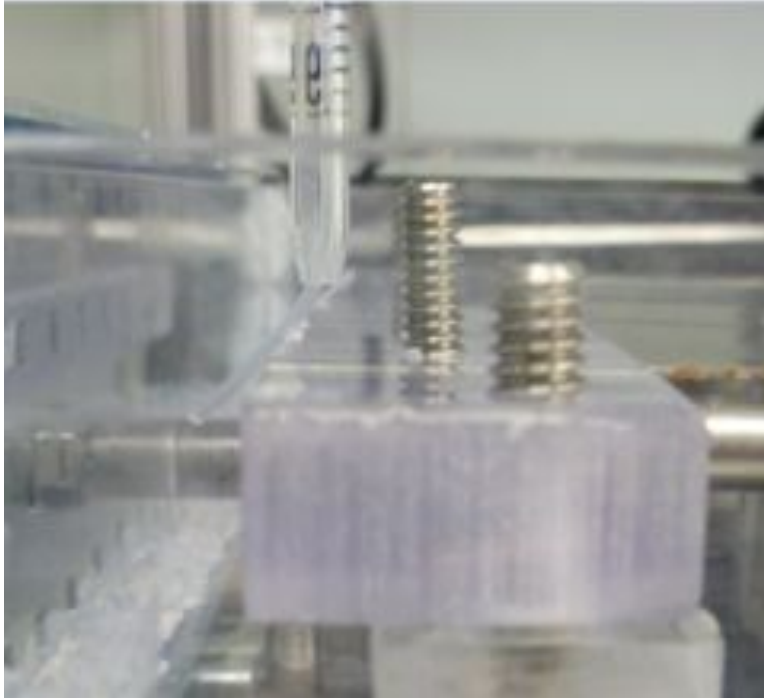
Figure 78: Position of polyethylene tubing - the polyethylene tubing sticking out of glass pipet should be 10 mm
