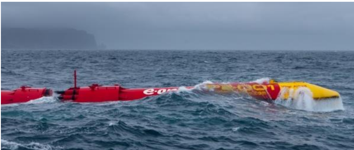
Figure 5-1: Pelamis Buoy Type Wave Power Generator [26]
