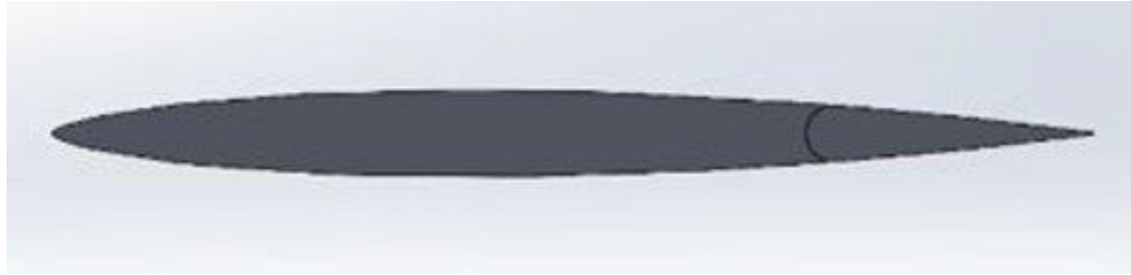
Figure 11: Side view of NACA 0008 airfoil at zero angle of attack modeled in Solidworks.
