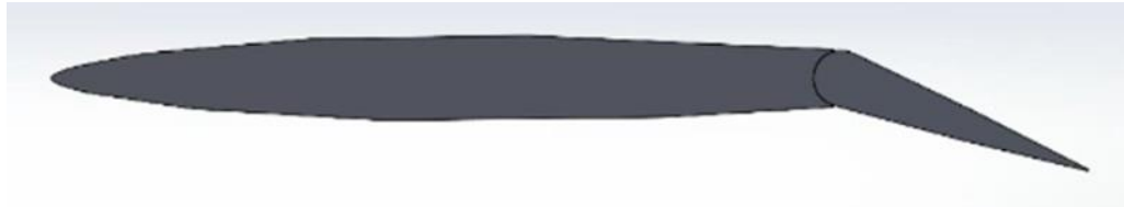
Figure 12: Side view of modified NACA 0008 airfoil with deflected elevator at zero angle of attack.
