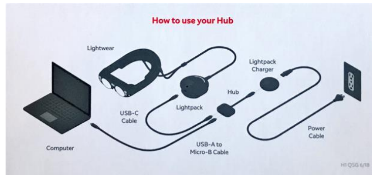
Figure 13. Magic Leap setup diagram 35 .
