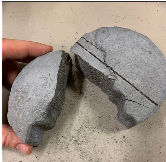
Figure 58: Top view of 3C after breaking at a 25 degree load angle. Within Mode II fracture, sample 3C broke at the highest load of 7,406 lbs. Sample 3C created an essentially
