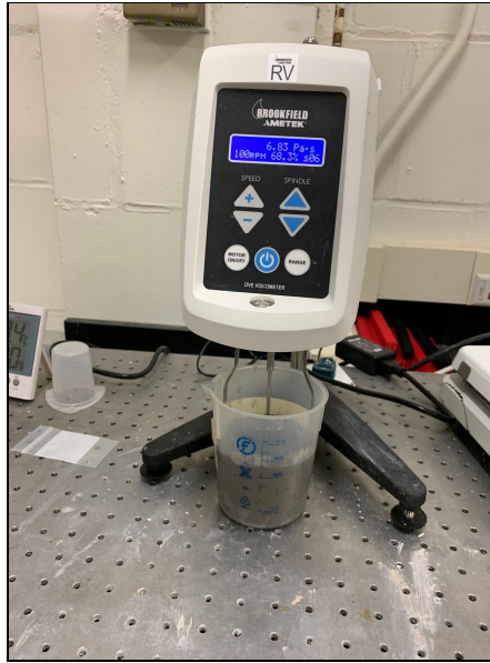
Figure 20: Image of the Brookfield viscometer with a concrete mix being measured.
