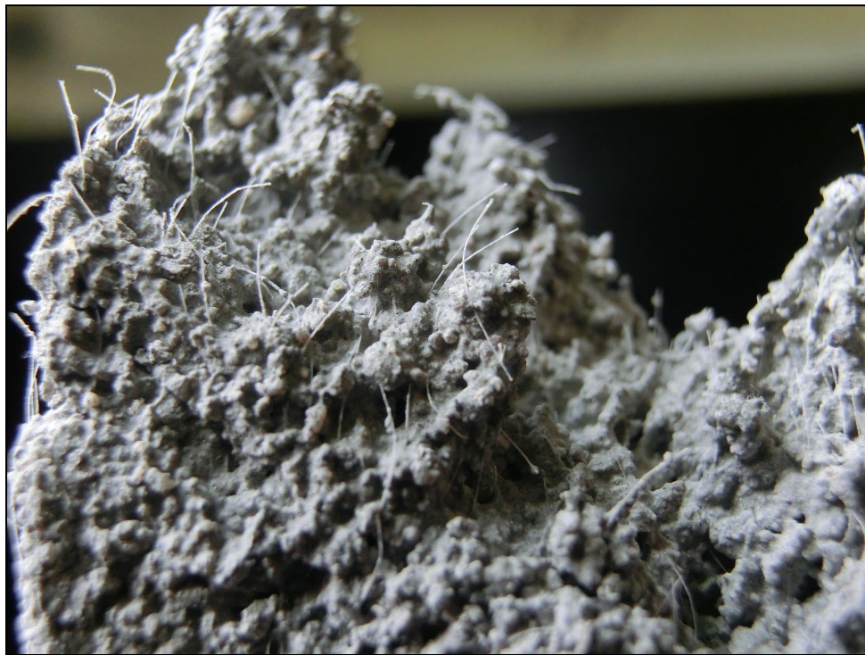
Figure 49: Macroscopic image of the end of a printed layer showing interior fibers also
