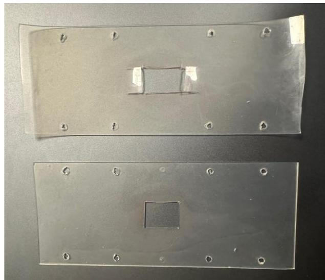
**Figure 63: Gaskets.** These silicone rubber gaskets were used to hold the membrane in place as well as provide a slope for the flow to ensure no large height differences.
