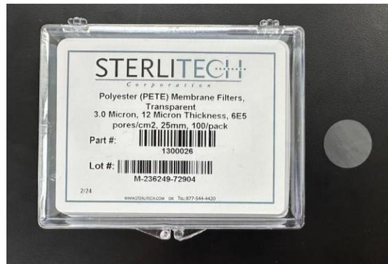
**Figure 64: Sterlitech PETE 3.0-Micron Membranes.** These are the membranes that were used in final testing because they met all the above qualifications and are biocompatible.
