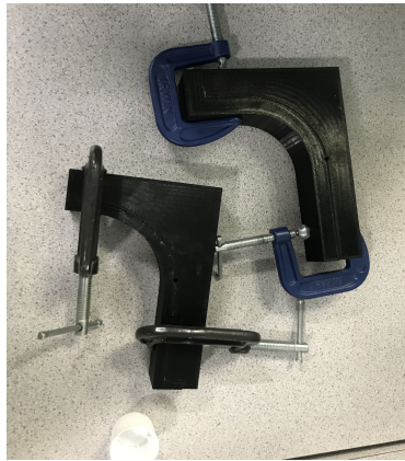
Figure 35: Mold Halves Clamped Together
