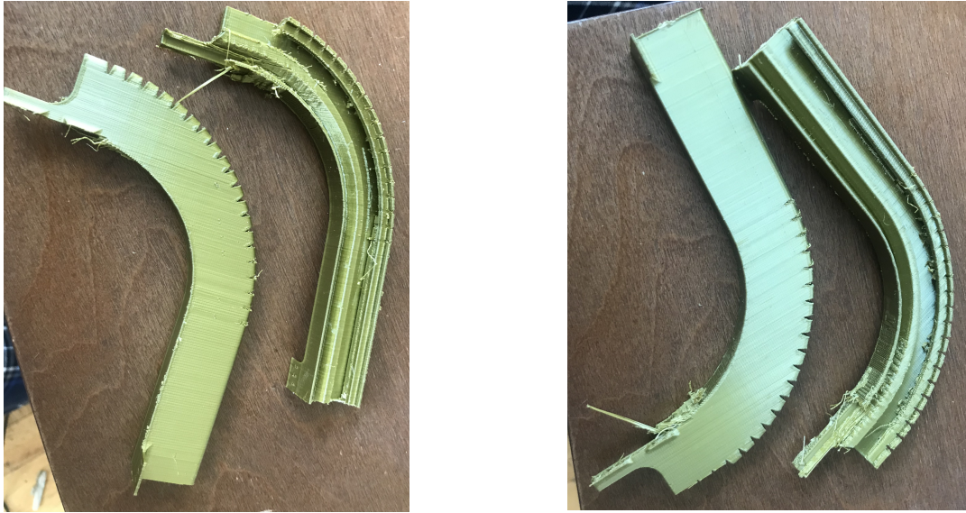
Figure 27: 3D Print Test of the Final Track Model
