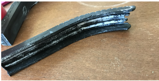
Figure 39: Top View of the Bottom Half of the Molded Pulley Track
