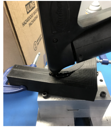
Figure 36: Mold Being Injected With the Gluco System
