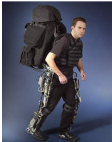
Figure 12: The BLEEX Device (Berkeley Robotics & Human Engineering Laboratory, n.d.)
