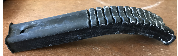
Figure 38: Top View of the Top Half of the Molded Pulley Track
