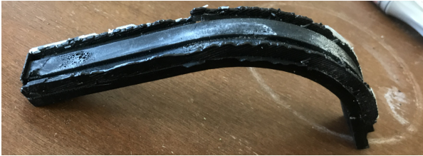
Figure 37: Top View of the Bottom Half of the Molded Pulley Track
