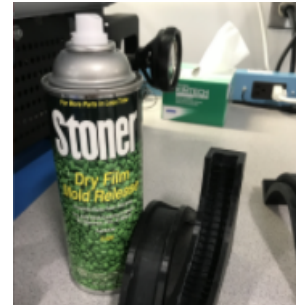
Figure 34: Spray Mold Release
