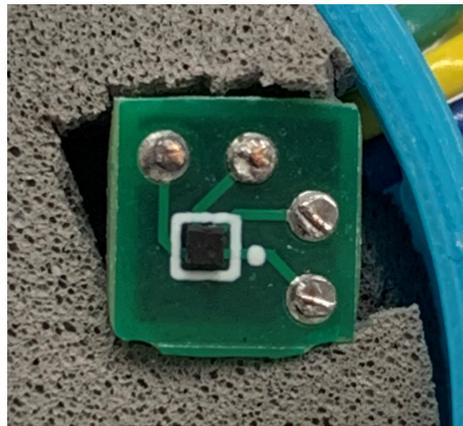
Figure 15: Analog sensor on PCB.
