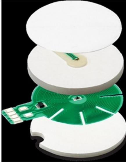
Figure 3: Prototype zero-heat flux sensor with two thermometers, an insulator, and a heater cover [9].
