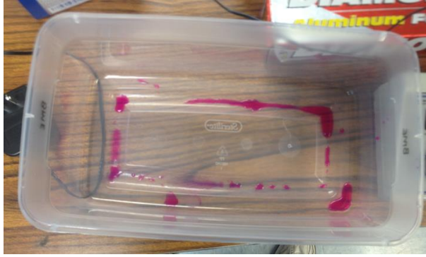
Figure 30: Leakage from sterility test
