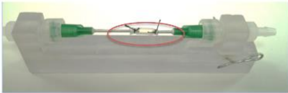
Figure 27: A view of the polycarbonate support piece and a mounted and sutured silicone tube, circled in red
