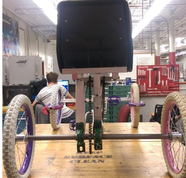
Figure 32: Rear of Lever Arm Drive System
