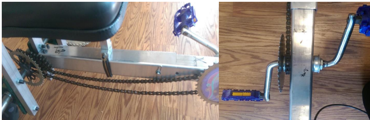
Figure 33: Final Direct Chain Drive
