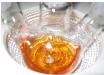
**Figure 13** – The quantum dot solution after the NaH<sub>2</sub>Te has been added to the Cd ion solution. The first was purple and the second colorless, together they formed an orange solution. Photo was taken directly after addition of NaH<sub>2</sub>Te, at the beginning of the growth of the quantum dots.
