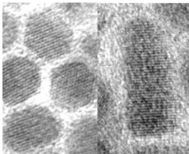
**Figure 3 – Quantum dots (left) and a quantum rod (right). (Peng, et al. 2000)**
