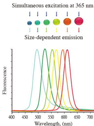
**Figure 2 – As the size of the quantum dots increases, so does the peak fluorescent wavelength. (Ooba 2006)**
