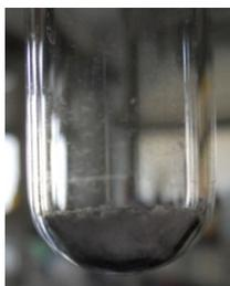
Figure 8 – Mixture of Te powder and  $\text{NaBH}_4$  powder before water was added.
