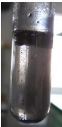
**Figure 9** – The Te powder and NaBH<sub>4</sub> mixture after pure water was added and the solution was shaken to mix.
