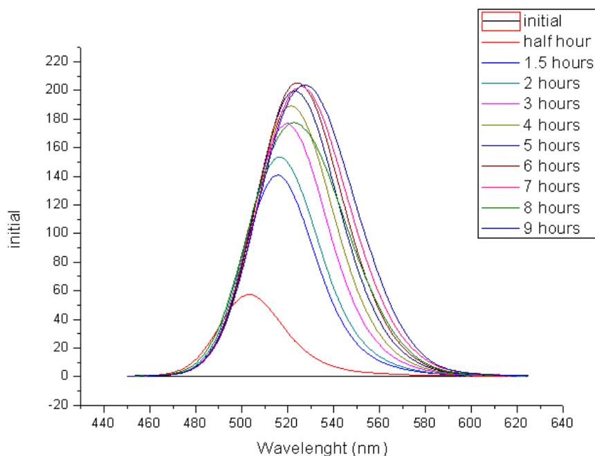
**Figure 22 – Fluorescence spectra for November 10<sup>th</sup> batch. (Taken on November 26<sup>th</sup>.) Note: the intensity of some of the samples was higher than the spectrometer could measure, resulting in a plateau instead of a peak, so the spectrums were redone at a lower light intensity.**
