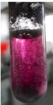
**Figure 10** – The NaHTe solution (purple) after ~24 hours in the refrigerator. Black sediment can be seen above and in the bottom of the solution.
