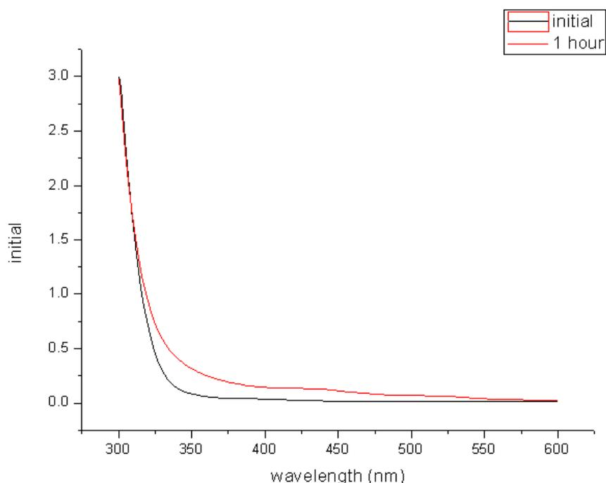
**Figure 15** – Graph showing absorption spectrums for initial and 1-hour sample from the batch made on October 29, 2010. (Spectrums were taken on November 12, 2010.)
