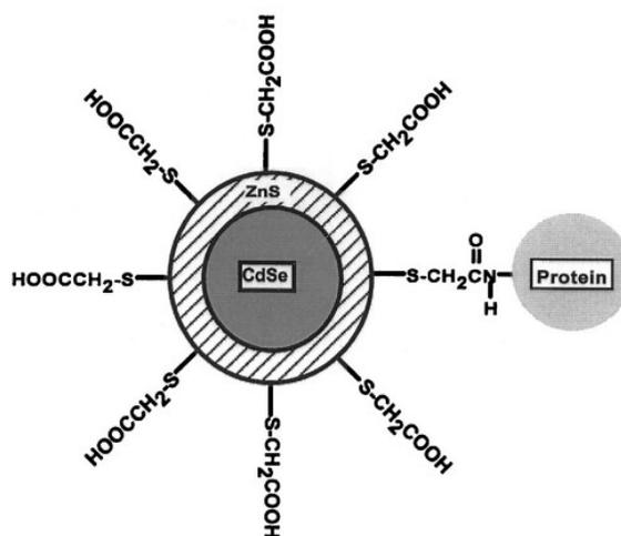
**Figure 1 – A quantum dot with two II-VI layers and capped by TGA, with a conjugated protein. (Chan and Nie 1998)**
