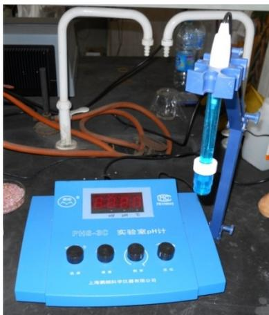
**Figure 5 - The pH meter used to adjust the pH in later experiments.**
