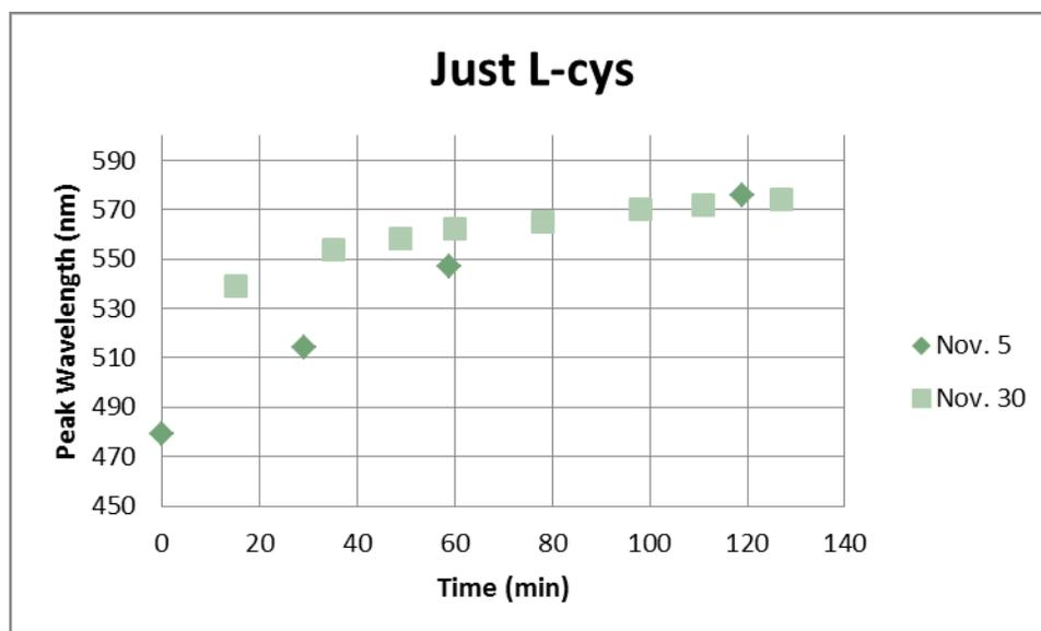
Figure 47 – Peak wavelength over time for batches grown using only L-cysteine.
