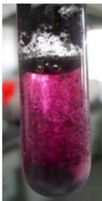
**Figure 10** – The NaHTe solution (purple) after ~24 hours in the refrigerator. Black sediment can be seen above and in the bottom of the solution.
