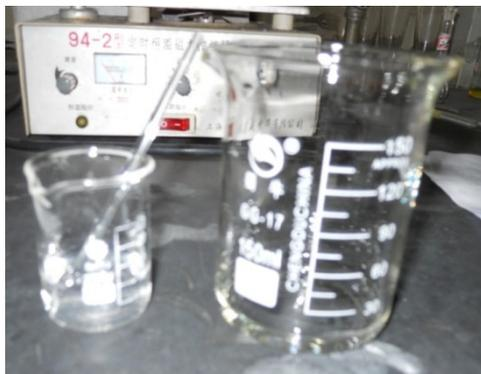
**Figure 11** – Dissolved L-cys (left beaker) and dissolved cadmium chloride (right beaker). Both were dissolved in pure water, and both are clear and colorless.
