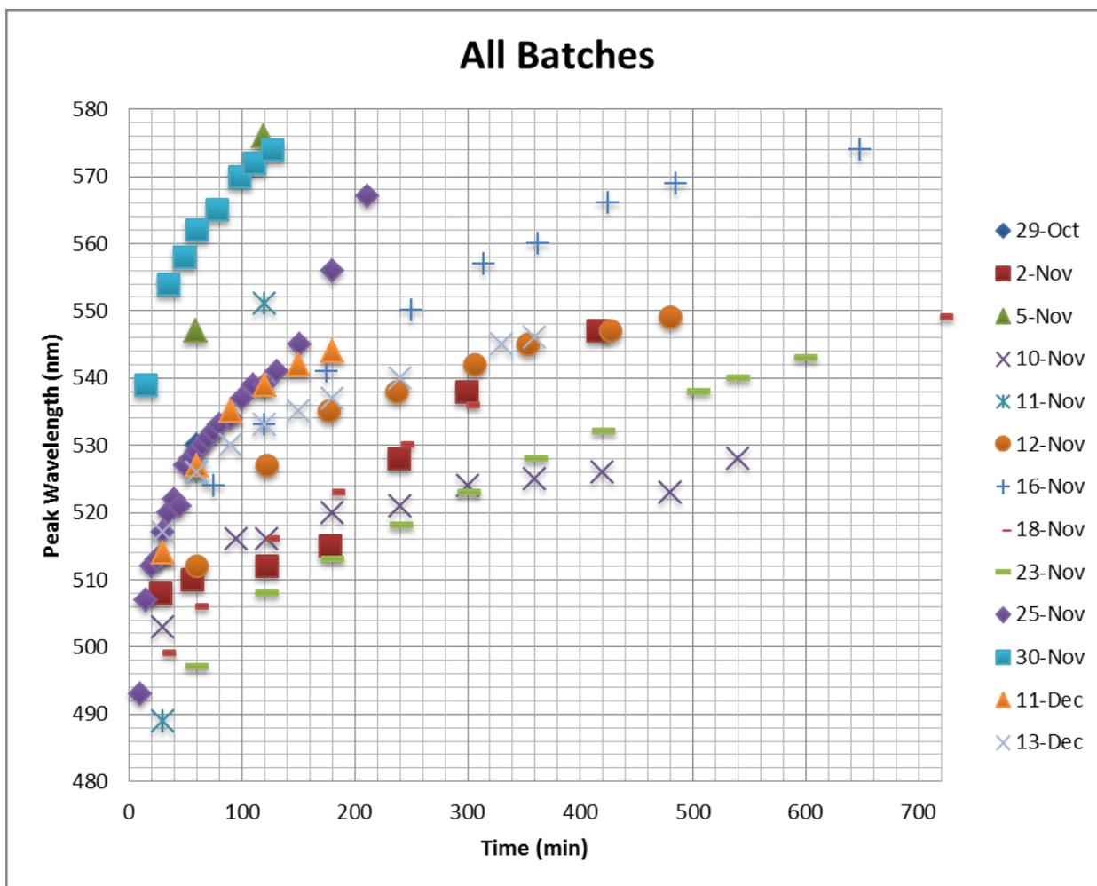
Figure 45 – Peak fluorescent wavelength over time (all quantum dot batches).
