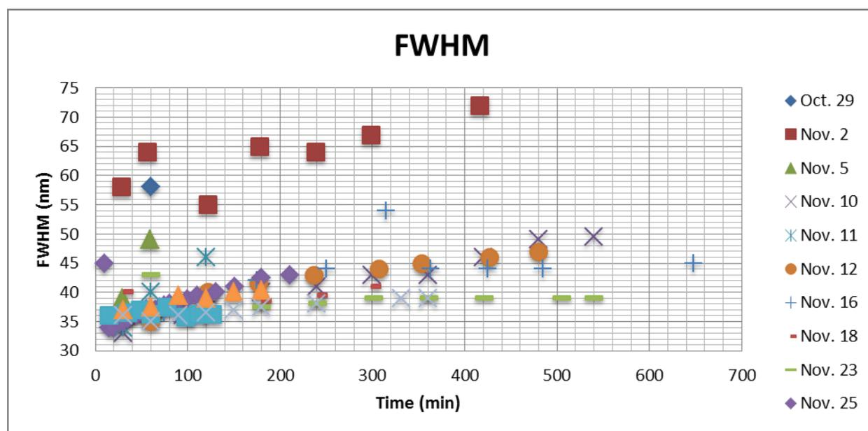
Figure 52 – Full width half maximum against sample time for all batches.
