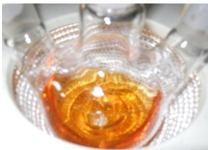
**Figure 13** – The quantum dot solution after the NaHTe has been added to the Cd ion solution. The first was purple and the second colorless, together they formed an orange solution. Photo was taken directly after addition of NaHTe, at the beginning of the growth of the quantum dots.
