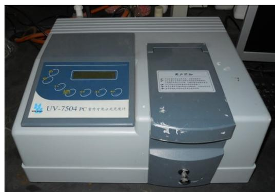
**Figure 6** - The absorption spectrometer.
