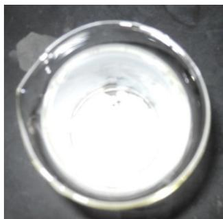
**Figure 12** – A white precipitate has formed in the Cd ion solution after the addition of a buffer.
