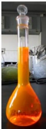
**Figure 14** – The 100 mL sample of rhodamine 6G. 0.1 mmol of r6G dissolved in ethanol. The solution appeared as a luminous orange, but stained paper and latex pink.
