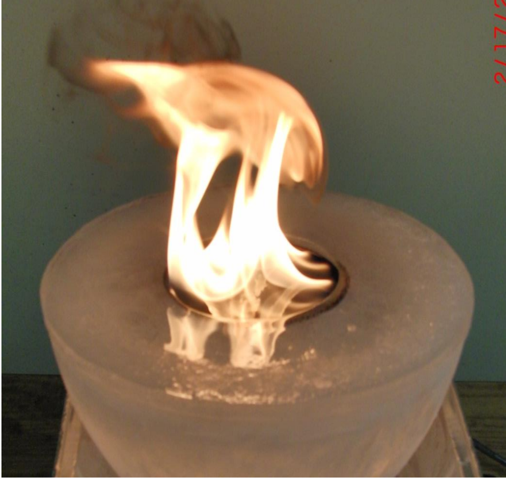
Figure B. 13: Burn test of Crude oil in 5 cm ice cavity- front view
