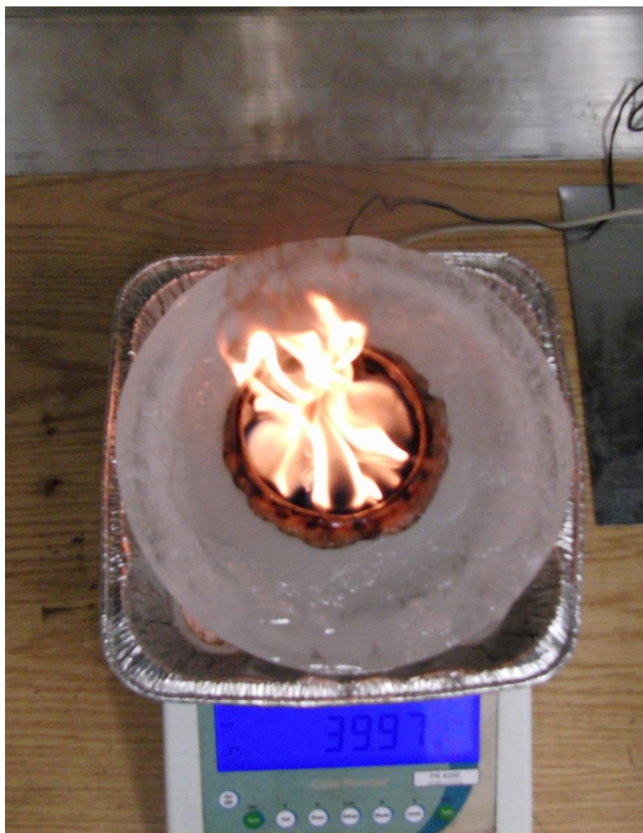
Figure B. 8: Burn test of Xylene in 5 cm ice cavity- top view
