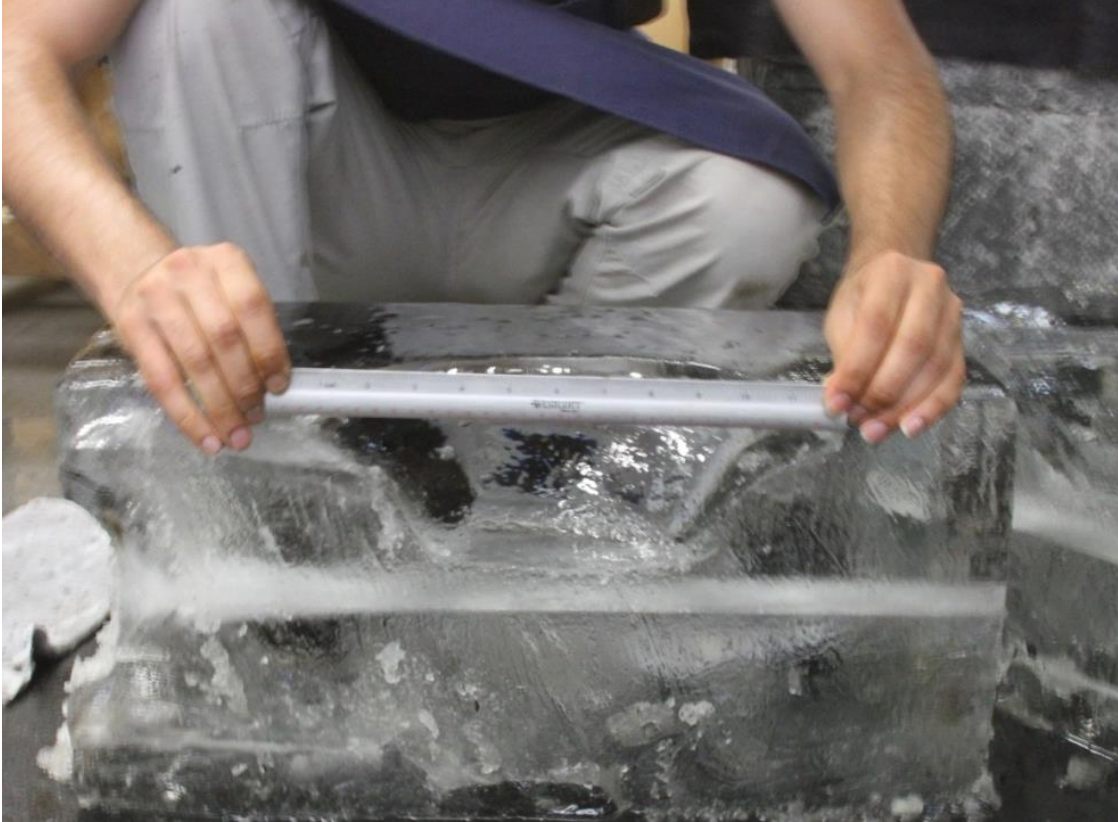
Figure B. 19: Cross section of the cavity after the extinction initial diameter of 15 cm
