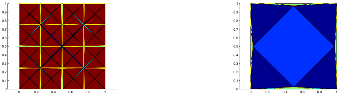
Figure 6.27: A classification of the domain into triangle types as \alpha \rightarrow 2 (left) and as \alpha \rightarrow 4 (right). The red toned area is the area covered by the matching triangles, whereas the blue toned areas are those covered by the slivers and center triangles.
