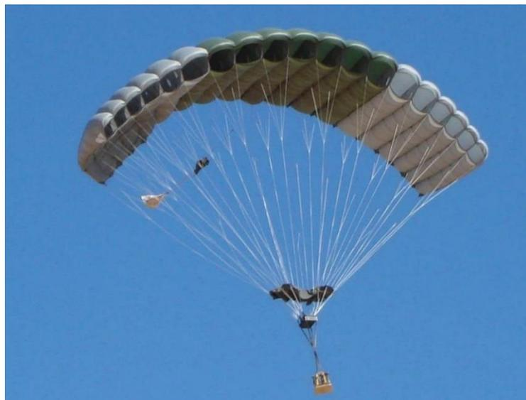
*Figure 1: DEVCOM uses parafoils to deliver supplies in areas that are difficult to reach otherwise. [5]*
