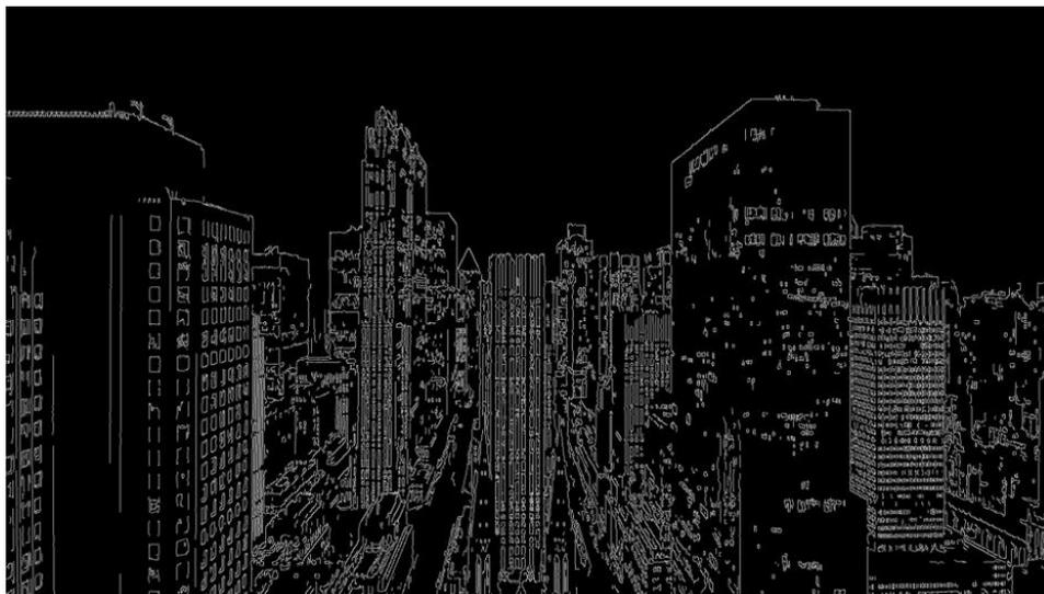
*Figure 20: Canny Edge Detection Applied on the Blurred Image*
