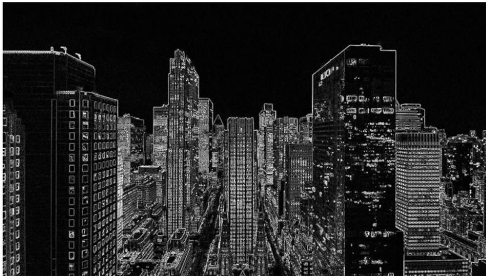
Figure 23: Laplacian Edge Detection applied on the Blurred Image
