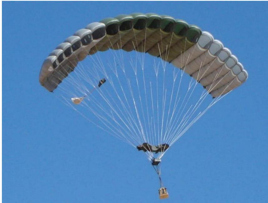
*Figure 2: The Joint Precision Airdrop System (JPADS) includes a parachute decelerator, an autonomous guidance unit and a load container. [5]*
