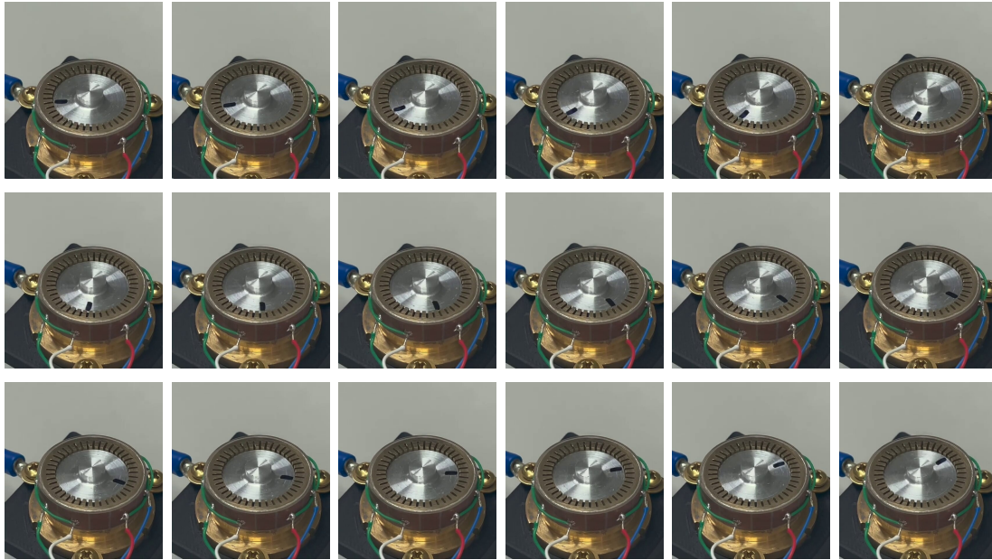
Figure 4.7: Rotor #2 Motion Captured Frame by Frame at 30.822 kHz and 900 mV p-p
