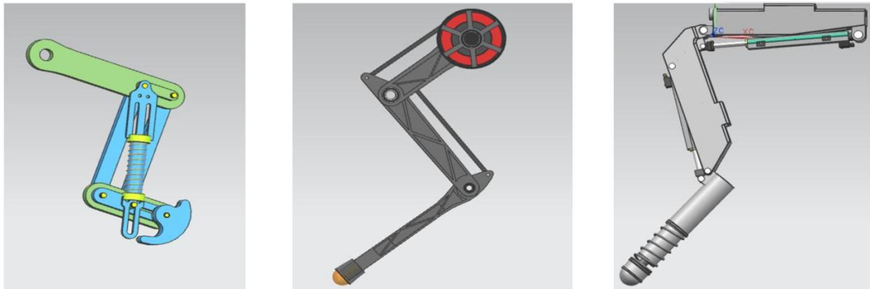
Figure 4: Preliminary leg designs (Cheetah 1, Cheetah 2, Dog)
