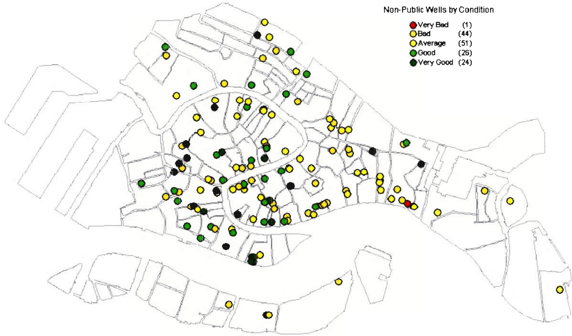
Figure 19: Wellhead damage assessment
