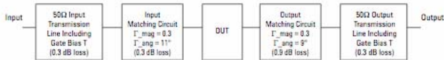
Figure 5. Block diagram of 2 GHz production test board used for Noise Figure, Gain, P1dB, OIP3, and IIP3 measurements. This circuit represents a trade-off between an optimal noise match, maximum OIP3 match and associated impedance matching circuit losses. Circuit losses have been de-embedded from actual measurements.
