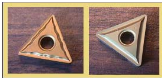
(d) Tools with Three-Dimensional Chip-Breaking Groove
