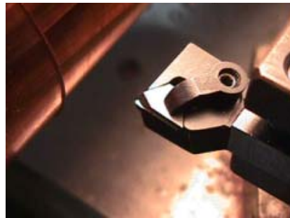
(b) Tool with Block Type Chip Breaker
