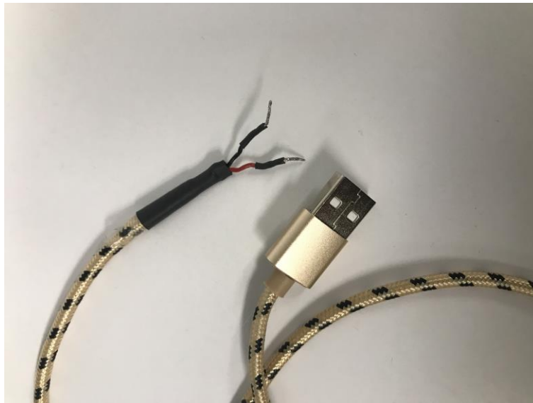
Figure 17. Power Cable-Modified for Breadboard
