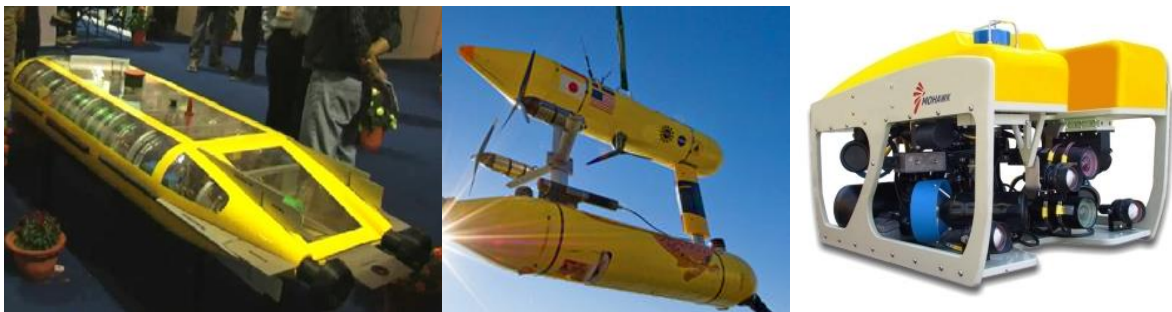
Figure 5: Pressure Vessel (left) [26], Flooded Shell (middle) [27] and Open Frame (right) [28] AUVs.
