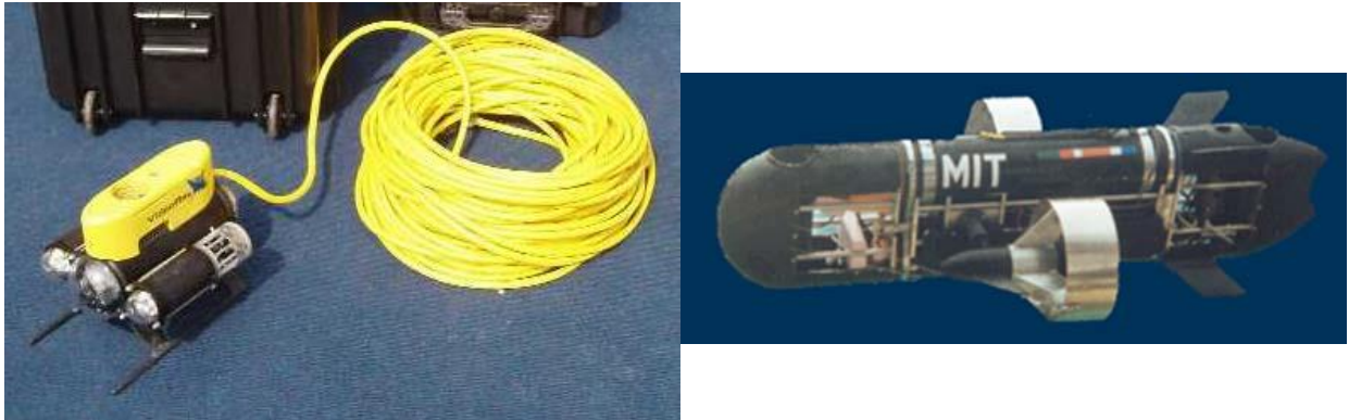
Figure 1: An ROV (left, has tether) [7] and AUV (right, no tether) [8]
