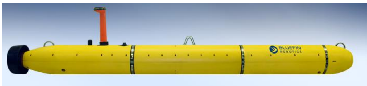
Figure 2: Bluefin-12S - A typical Torpedo Shaped AUV [18]
