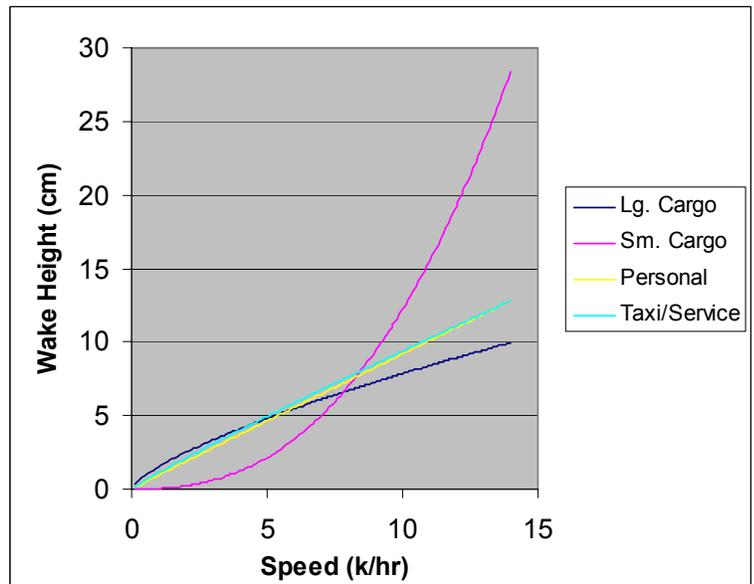
Figure 4-6 Regression Plots of Speed vs. Wake Height for Different Boat Types
