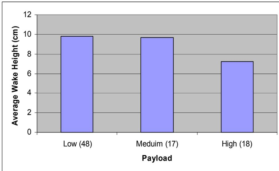
Figure 4-9 Average Wake Size of Large Cargo Boats with Different Payloads
