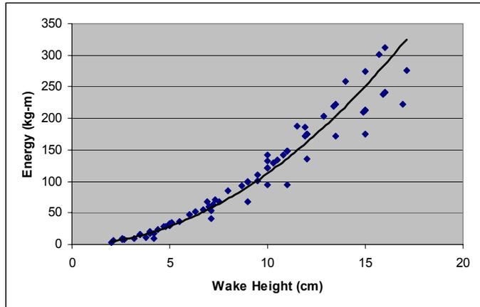
Figure 4-11 Wake Height vs. Energy for Large Cargo Boats
