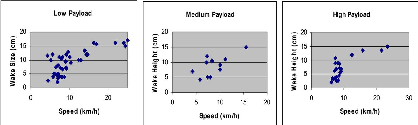
Figure 4-8 Speed vs. Wake size of Large Cargo Boats with Different Payloads
