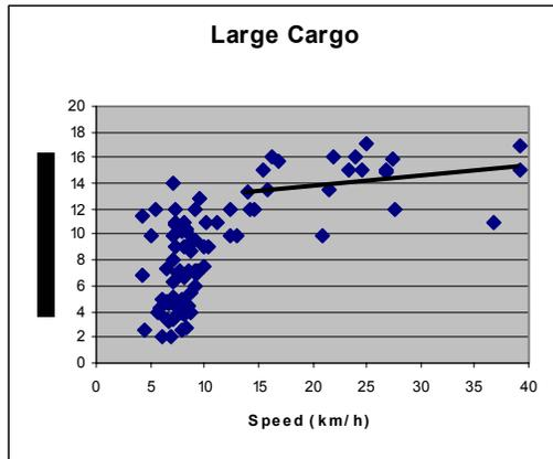
Figure 4-7 Regression of Speed vs. Wake Height for Large Cargo Boats Traveling Above 14 km/h
