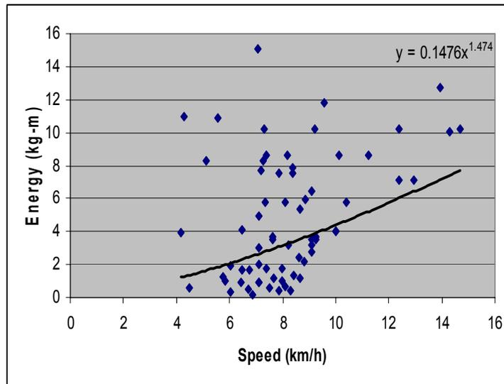
Figure 4-12: Velocity vs. Energy for Large Cargo Boats
