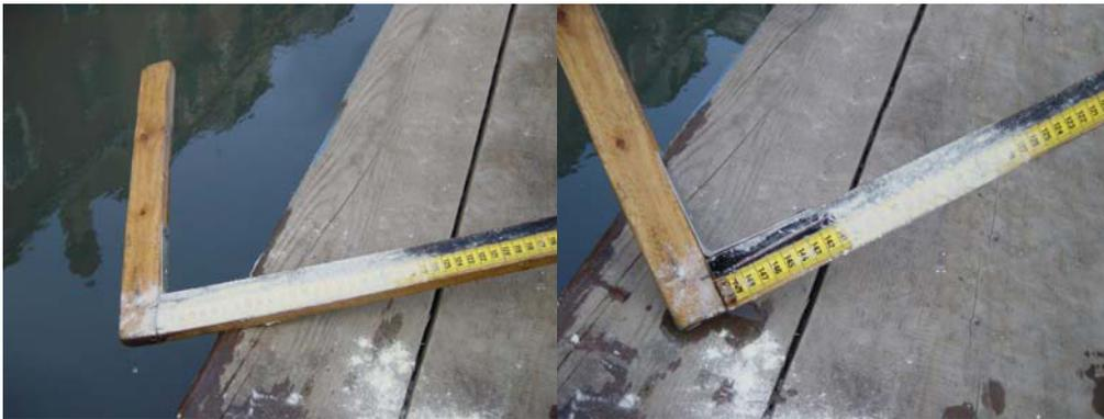
Figure 3-6: The wake measuring device before and after measuring a boat's wake
