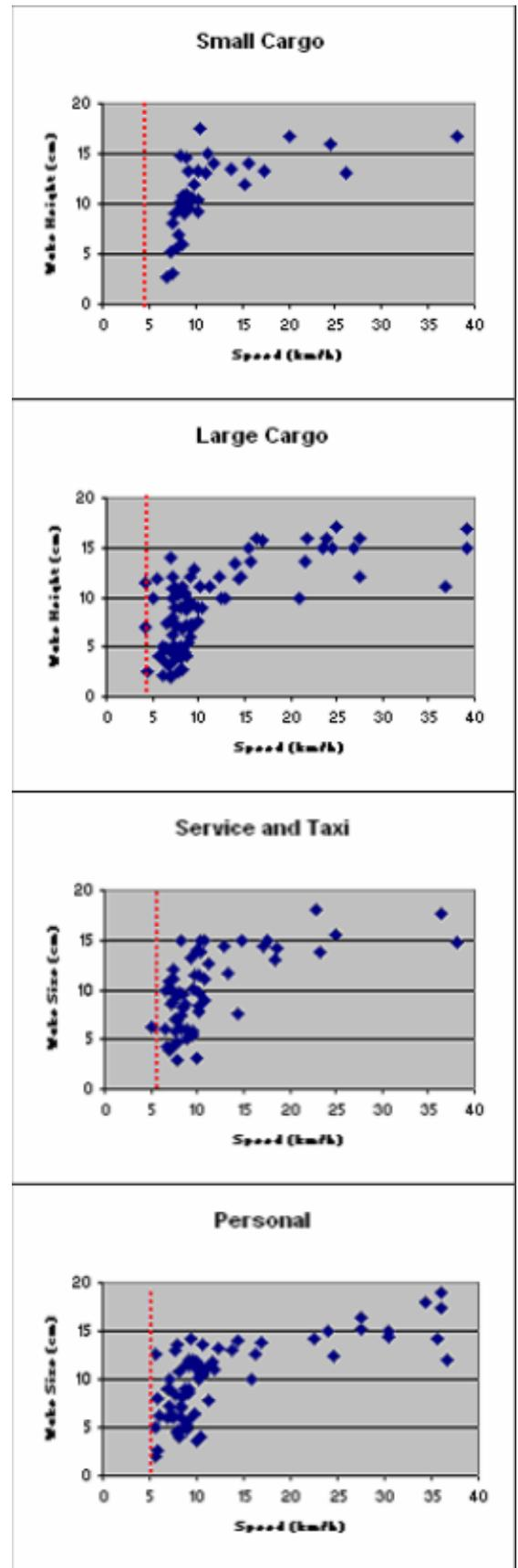
Figure 4-4 Speed vs. Wake Height for Different Boat Types
