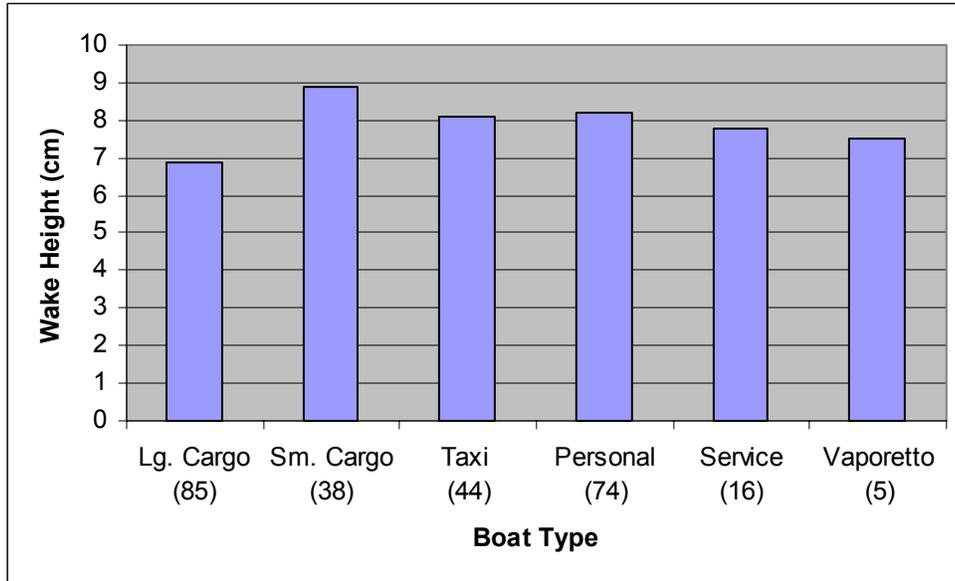
Figure 4-5 Average Wake Sizes of Different Boat Types Traveling Between 5 km/hr and 10 km/h
