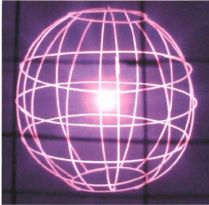
Figure 3 - Image of the D+ 3 He reactor from the University of Wisconsin
