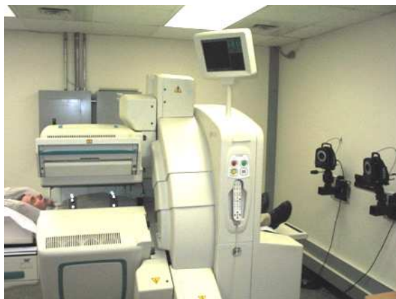
Figure 1.4: Illustration of viewing geometry for markers on stretchy bands and a volunteer in the supine position for motion-tracking during SPECT imaging.
