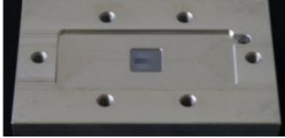
Figure 4: Mold tool with master placed at center
