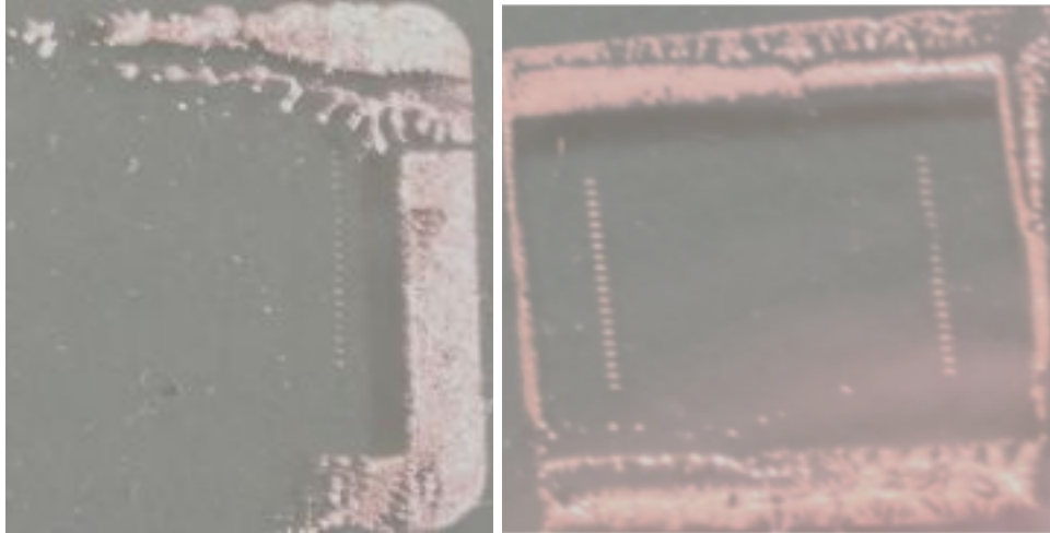
Figure 21: Visual print comparison [unacceptable (left) vs. acceptable (right)]
