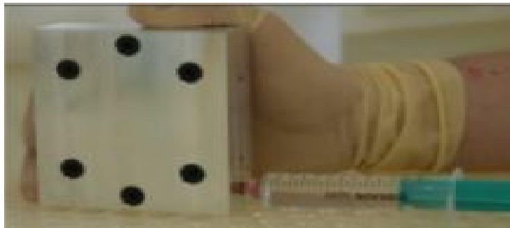
Figure 5: Closed mold tool being filled with PDMS
