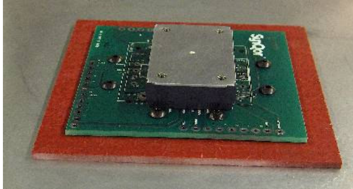
Figure 10: product and product test board assembly
