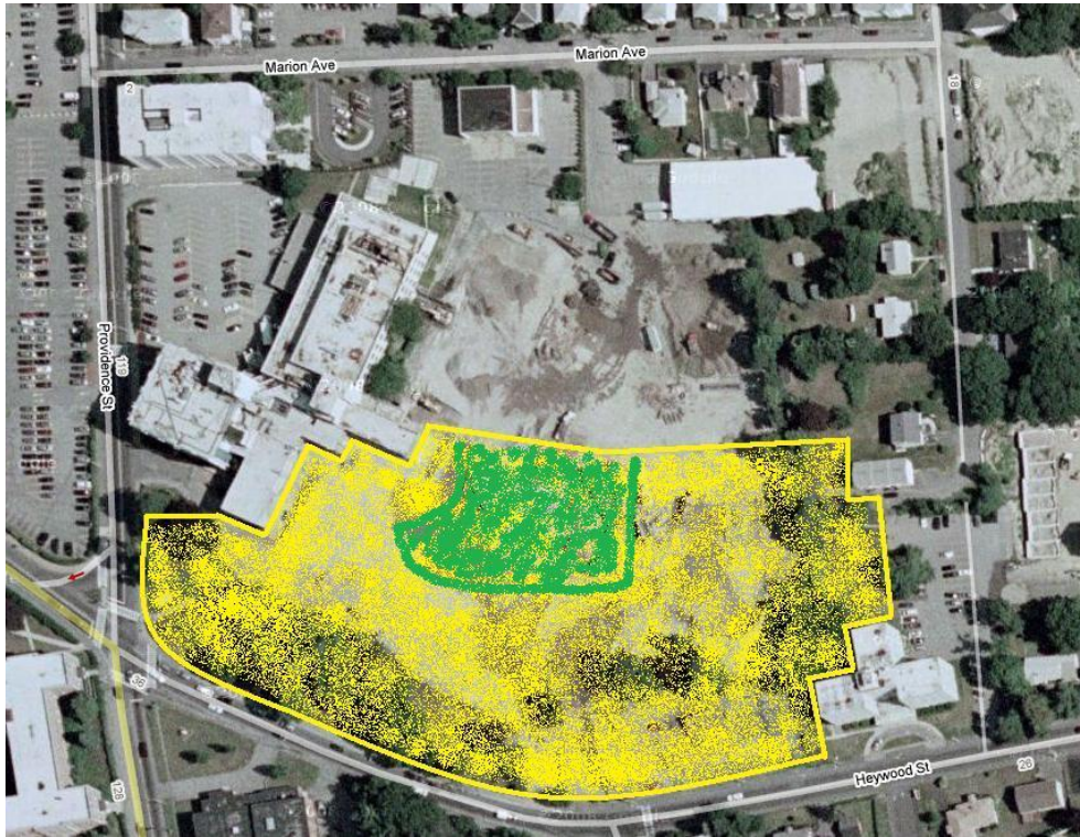
Figure 12: Allowable Location of Turbine Shaded in Green
